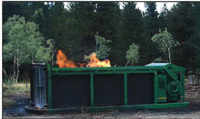
FireBox—No visible PM discharge
