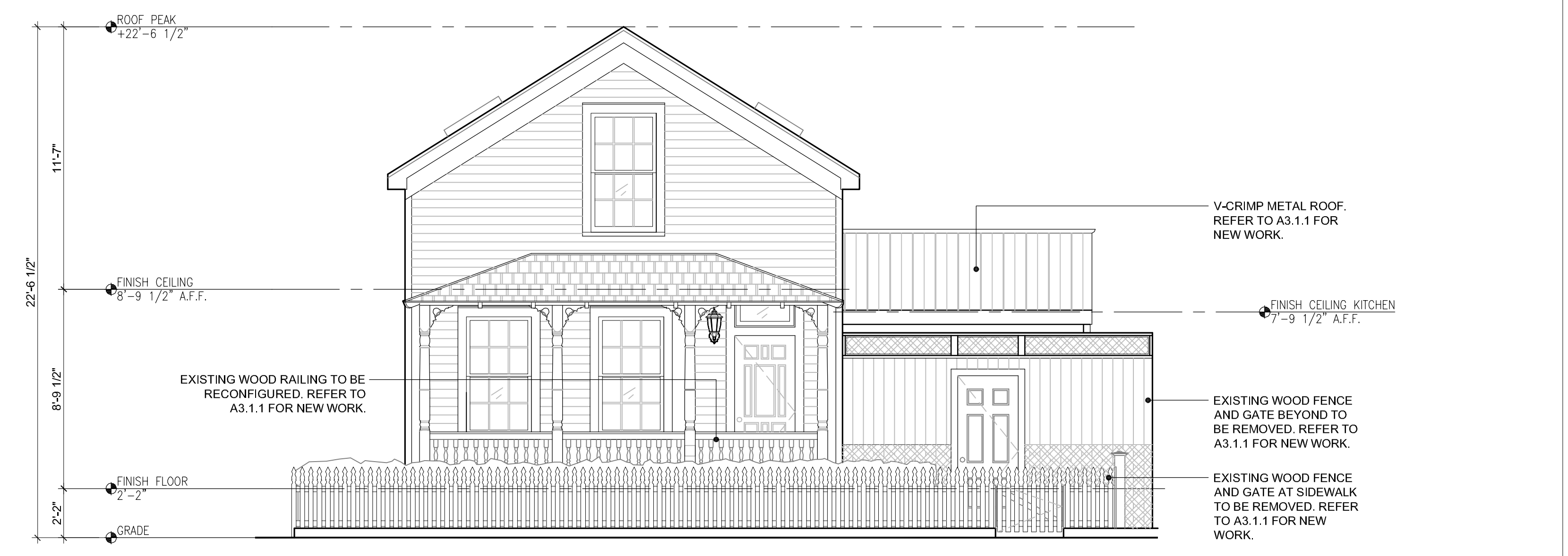
1 NORTH ELEVATION FROM STREET SCALE: 1/4"=1'-0"
