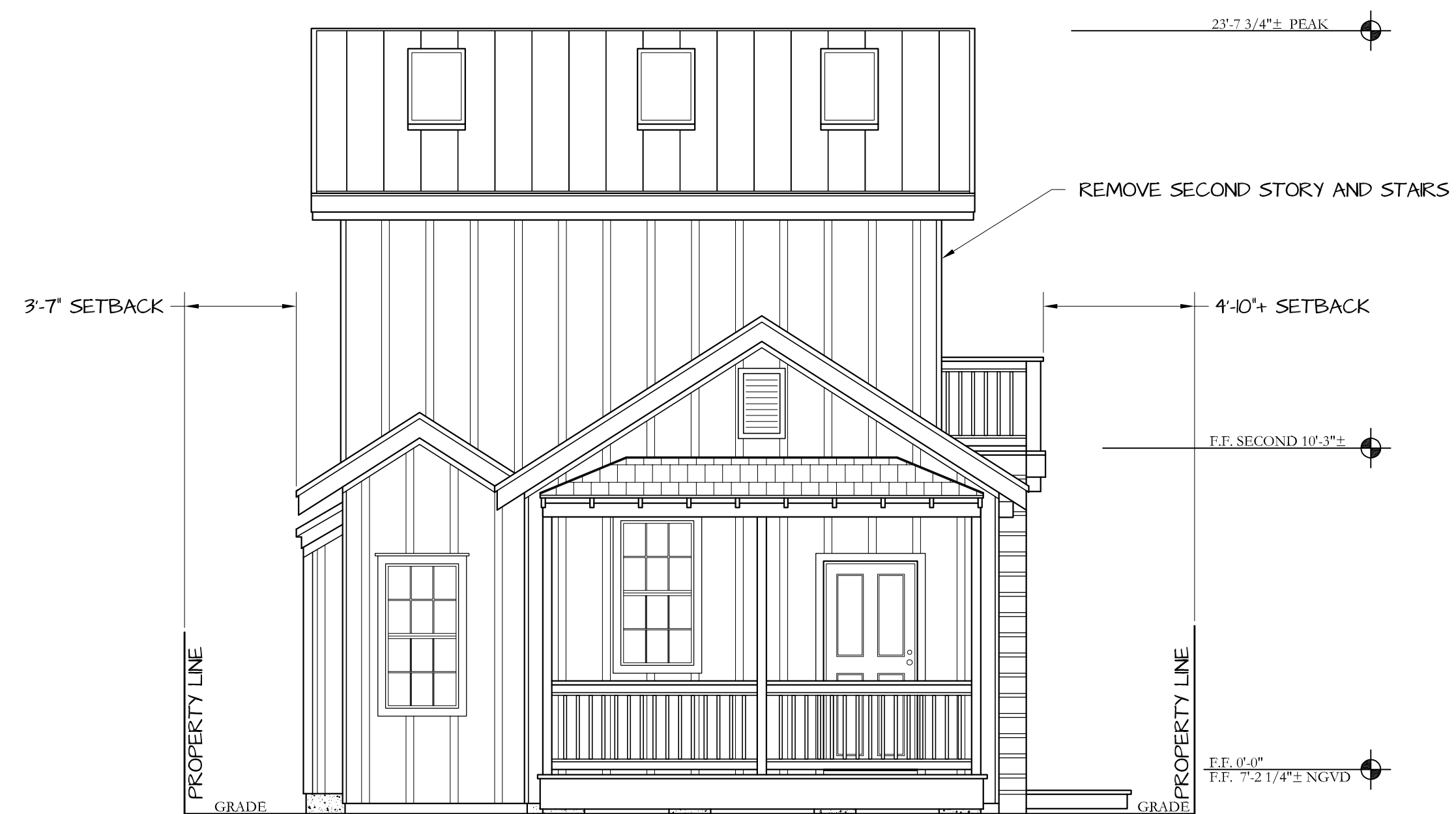
NORTH ELEVATION (EXISTING) 1/4" = 1'-0"
