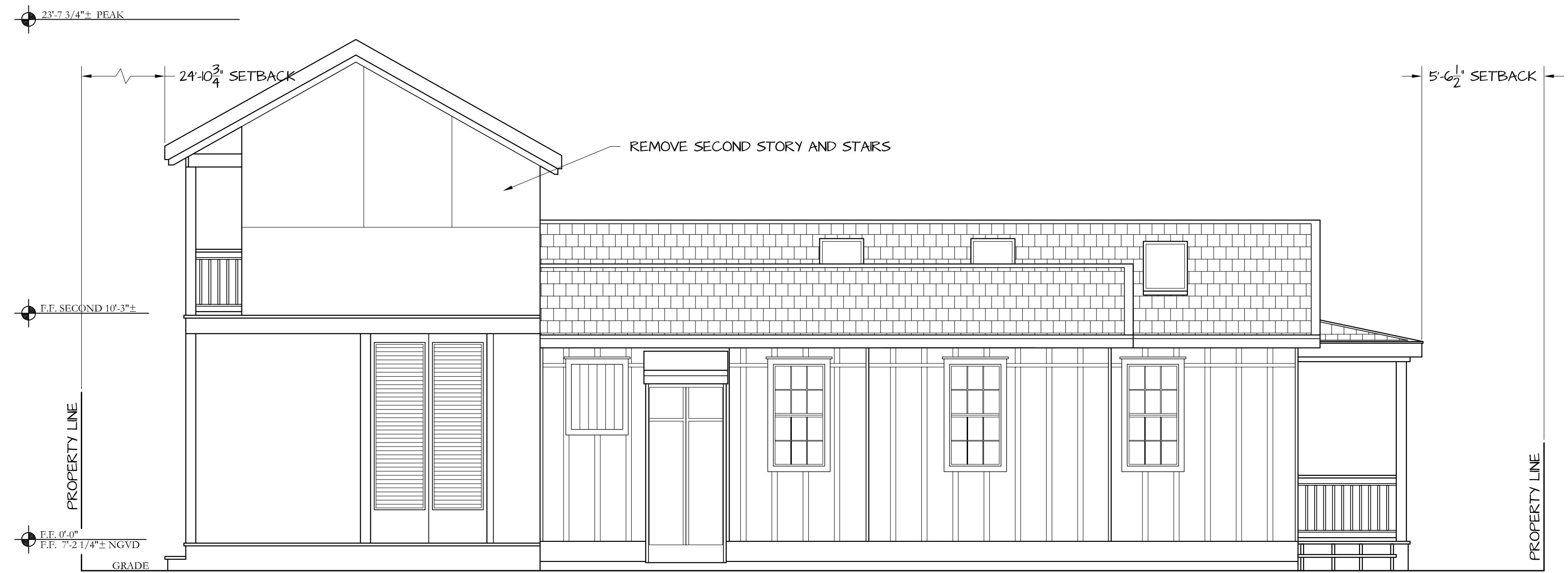
EAST ELEVATION (EXISTING) 1/4" = 1'-0"
