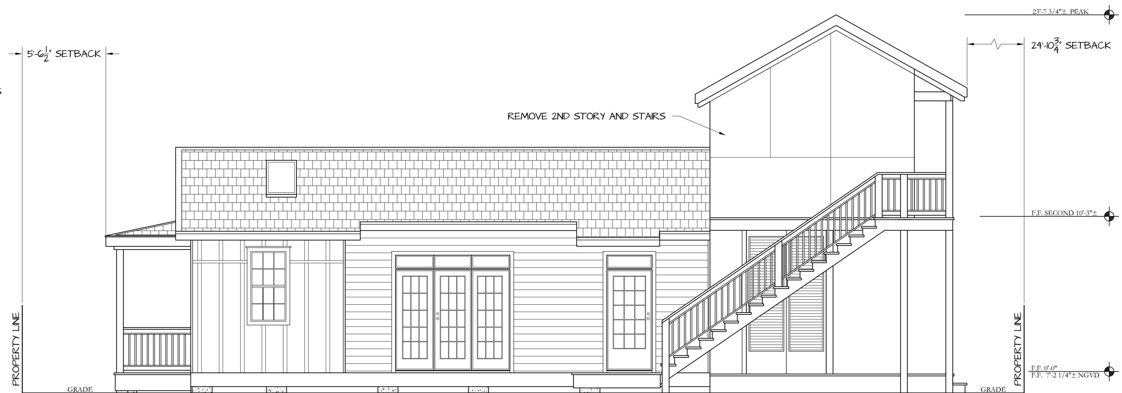
WEST ELEVATION (EXISTING) 1/4" = 1'-0"
