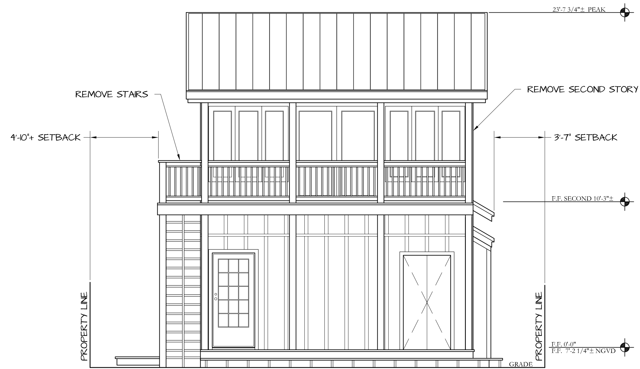
SOUTH ELEVATION (EXISTING) 1/4" = 1'-0"
