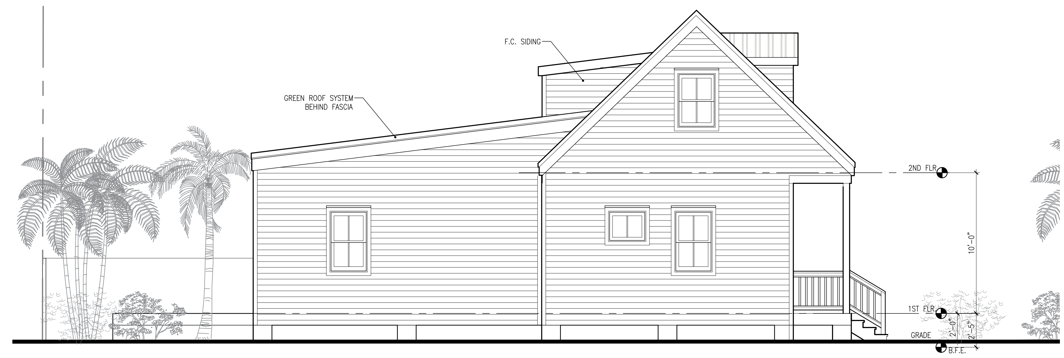
4 EAST ELEVATION SCALE: 1/4"=1'-0"
