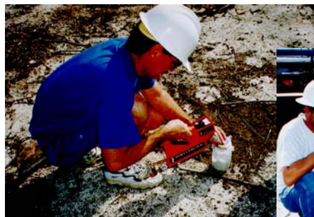
Test well drilling and soil testing for fuel tank removal and closure, Robbie's Marina, Stock Island
