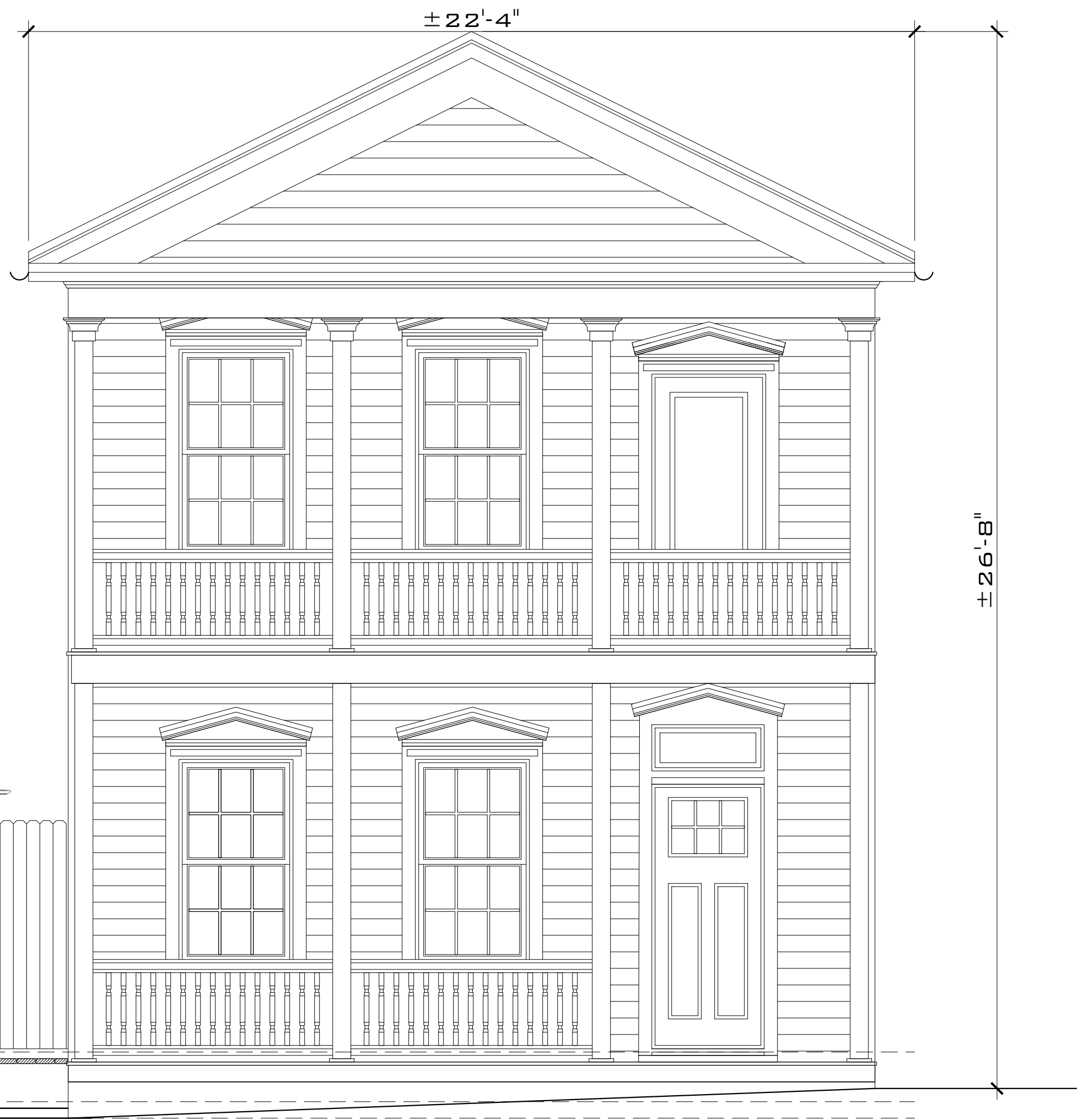
PROPOSED FRONT ELEVATION SCALE: 3/8" = 1'-0"
