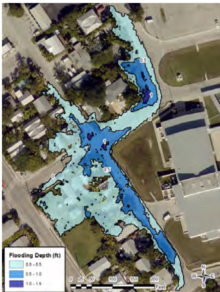
This is a visualization of predicted inundation from a two-dimensional modeling in XP-SWMM for the Dennis Street Stormwater Improvements Project. This project will alleviate flooding issues at the Key West High School.
