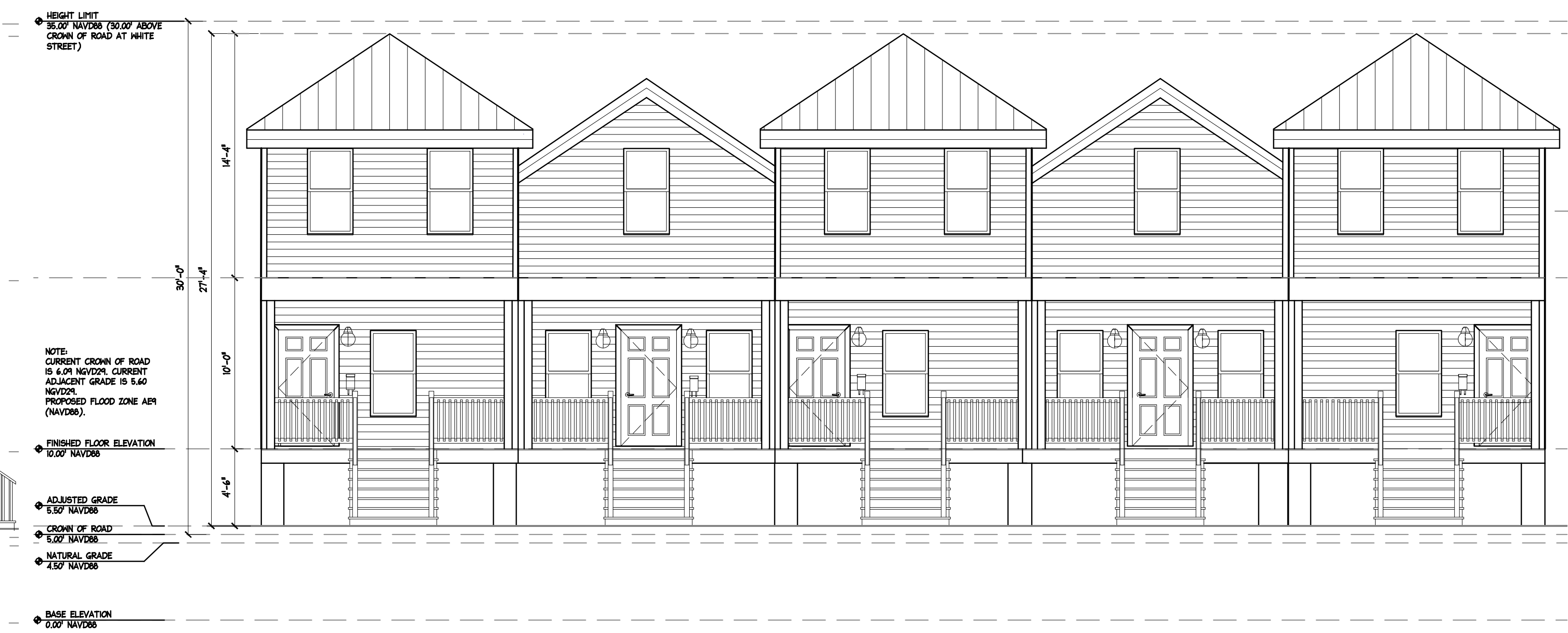
1 QUINTUPLEX FRONT ELEVATION (SITE #9) SCALE: 3/16"=1'-0"
