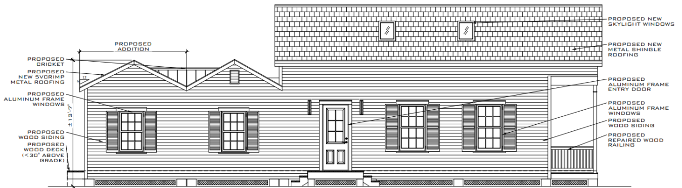
PROPOSED LEFT ELEVATION SCALE: 3/8" = 1'-0"
