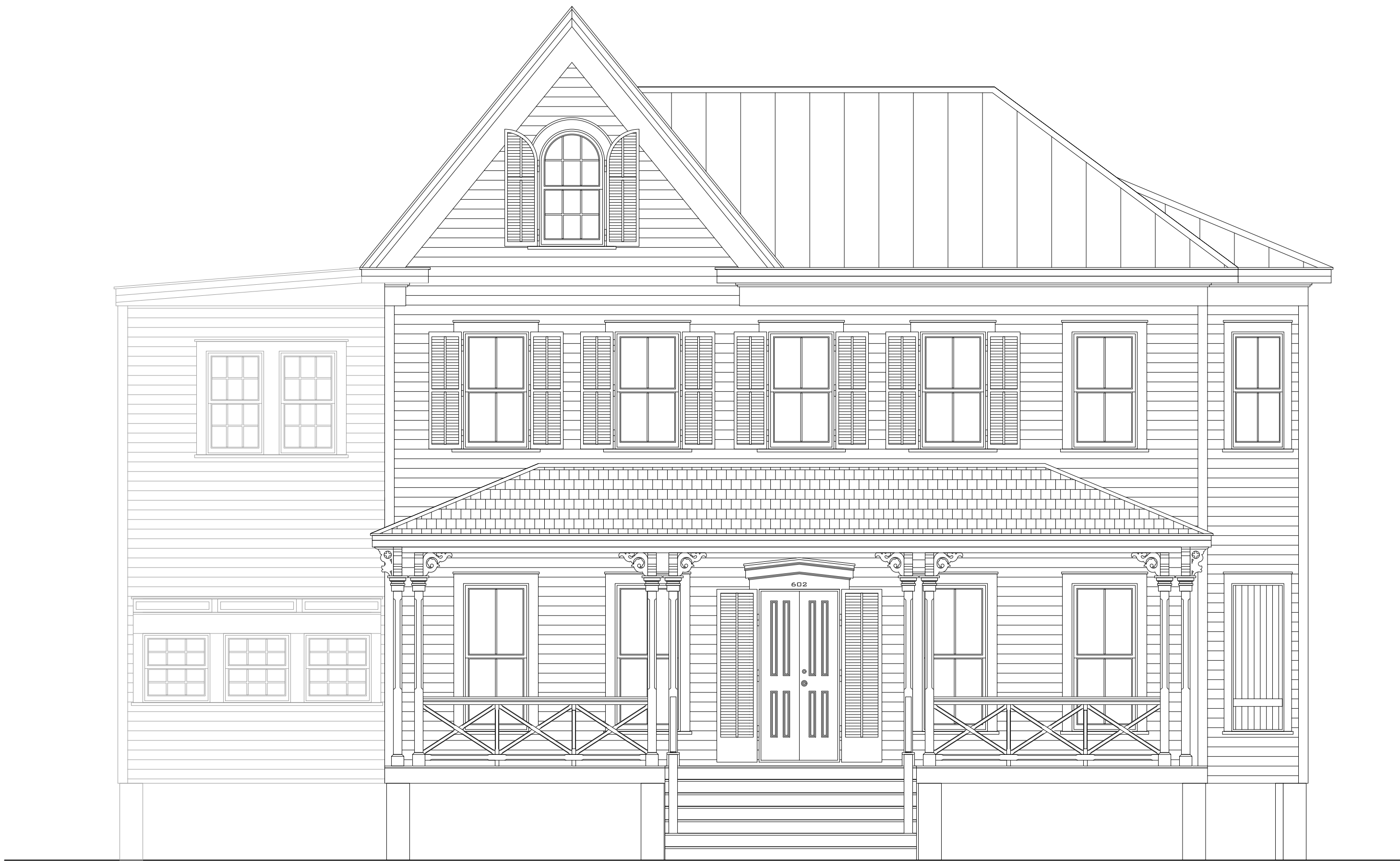
EXISTING FRONT ELEVATION SCALE: 1/4" = 1'-0"
