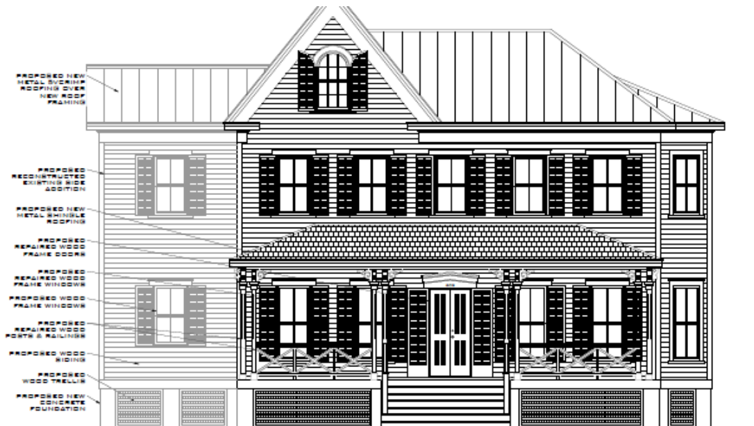
PROPOSED FRONT ELEVATION Scale: 1/4" = 1'-0"
