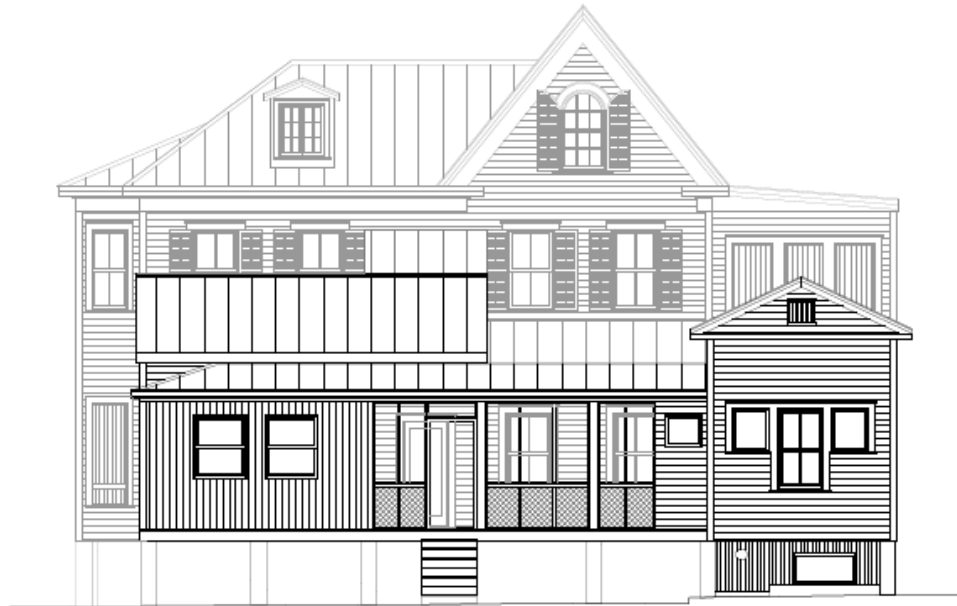
EXISTING REAR ELEVATION Scale: 1/4" = 1'-0"
