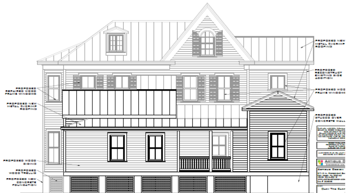
PROPOSED REAR ELEVATION Scale: 1/4" = 1'-0"
