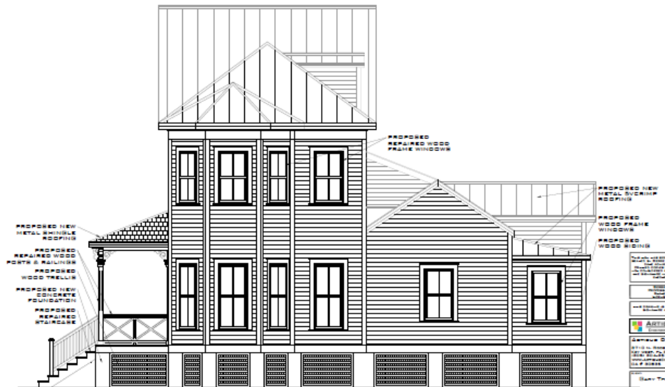
PROPOSED RIGHT ELEVATION SHEET 10 OF 10
