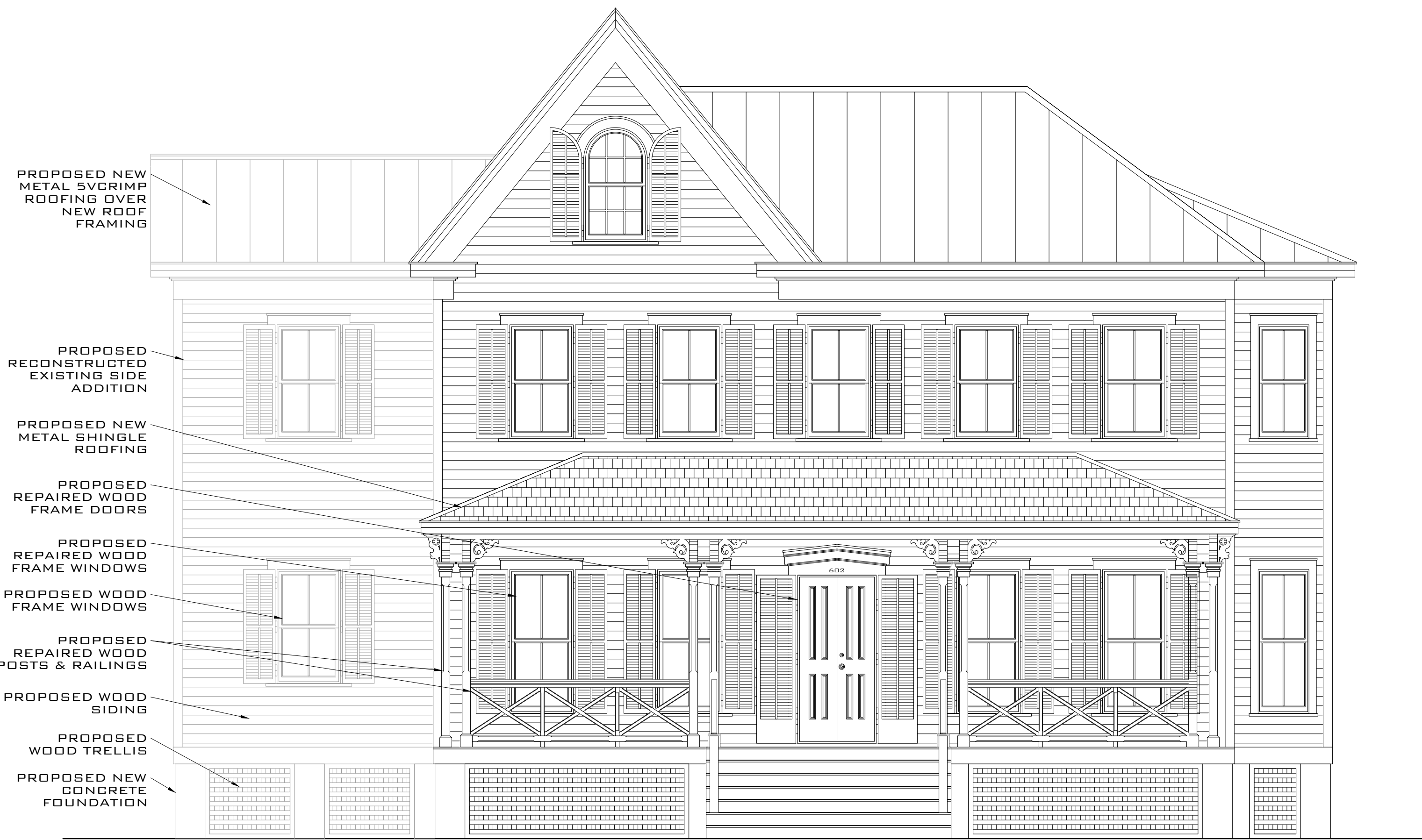
PROPOSED FRONT ELEVATION SCALE: 1/4" = 1'-0"
