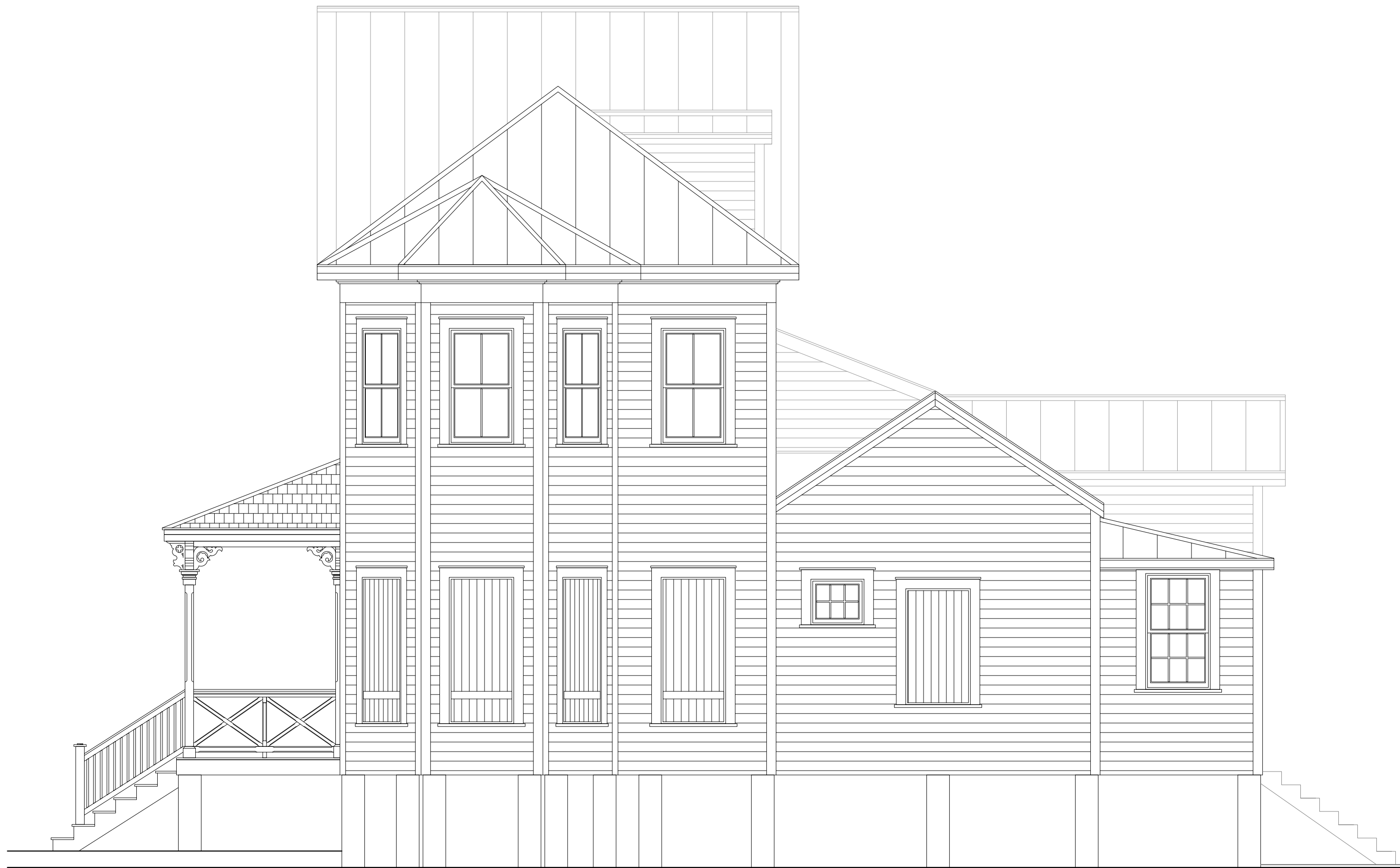
EXISTING RIGHT ELEVATION SCALE: 1/4" = 1'-0"
