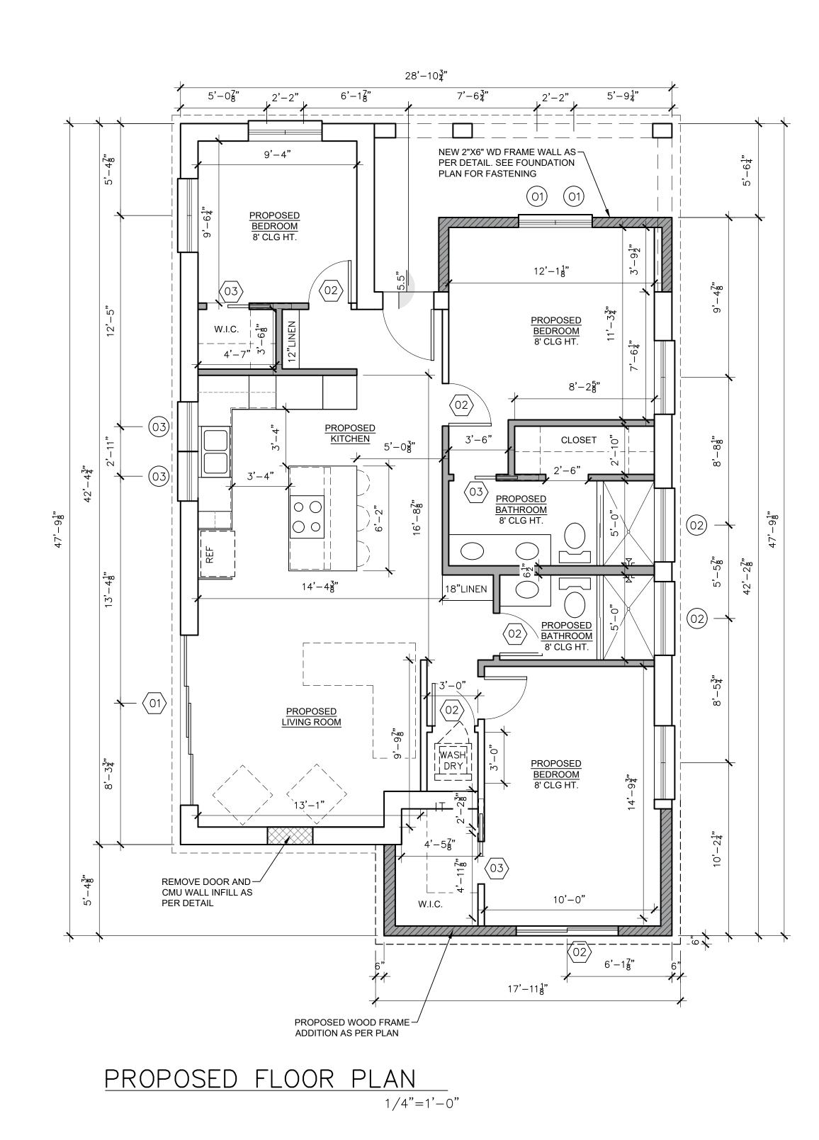
NOTE: ALL BEDROOMS SHALL HAVE AT LEAST ONE WINDOW OR DOOR THAT MEETS FL. BLDG. CODE 2023 FOR EGRESS. A MIN. 5.7 SQ. FT. NET CLEAR OPENING IS REQUIRED WITH A MIN. NET CLEAR HEIGHT OF 24" & MIN. NET CLEAR WIDTH OF 20" AND A SILL THAT IS NOT MORE THAT 44" AFF. ADDITIONAL NOTES:
