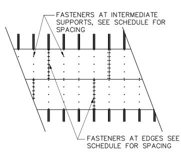
ROOF & WALL NAILING REQUIREMENTS SCALE = N.T.S.
