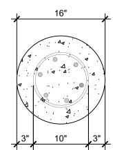
16" DIA CONCRETE AUGERCAST PILE W/ (6) #6 VERTICAL BARS & # 3 TIES @ 10" O.C. 3' INTO ROCK. CLEAN HOLES BEFORE PLACING 5,000 PSI CONCRETE
