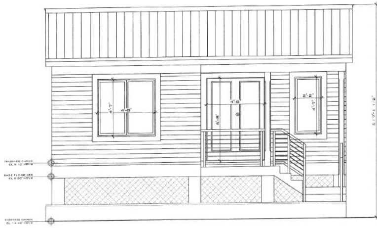
POOL SIDE ELEVATION SCALE: 1/4" = 1'-0"
