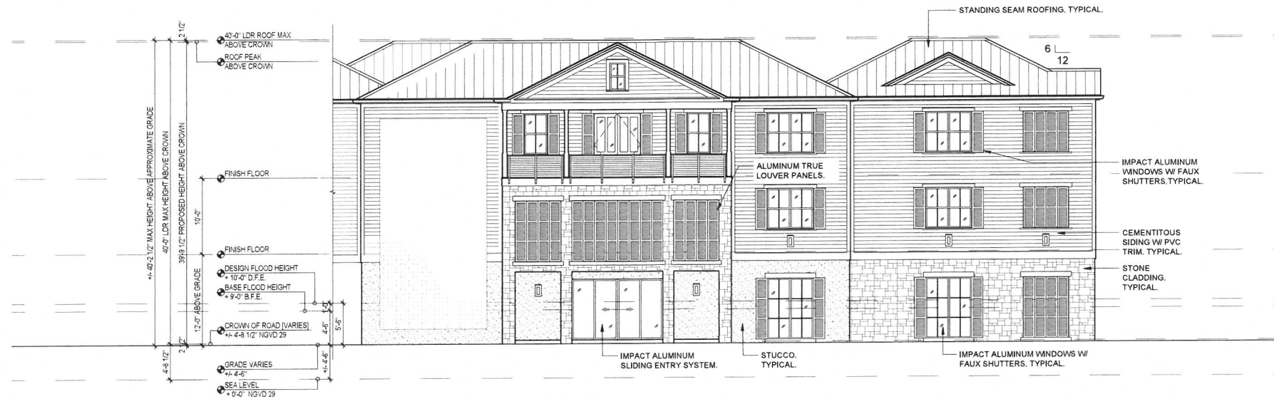
2 HOTEL LOBBY BUILDING: WEST ELEVATION [SIGSBEE] SCALE: 1/8"=1'-0"
