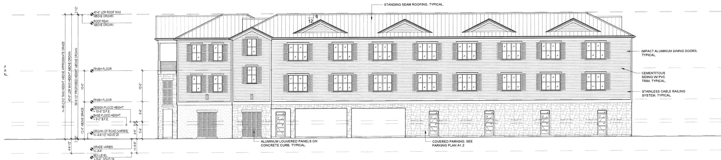
1 HOTEL LOBBY BUILDING: SOUTH ELEVATION [NORTH ROOSEVELT] SCALE: 1/8"=1'-0"
