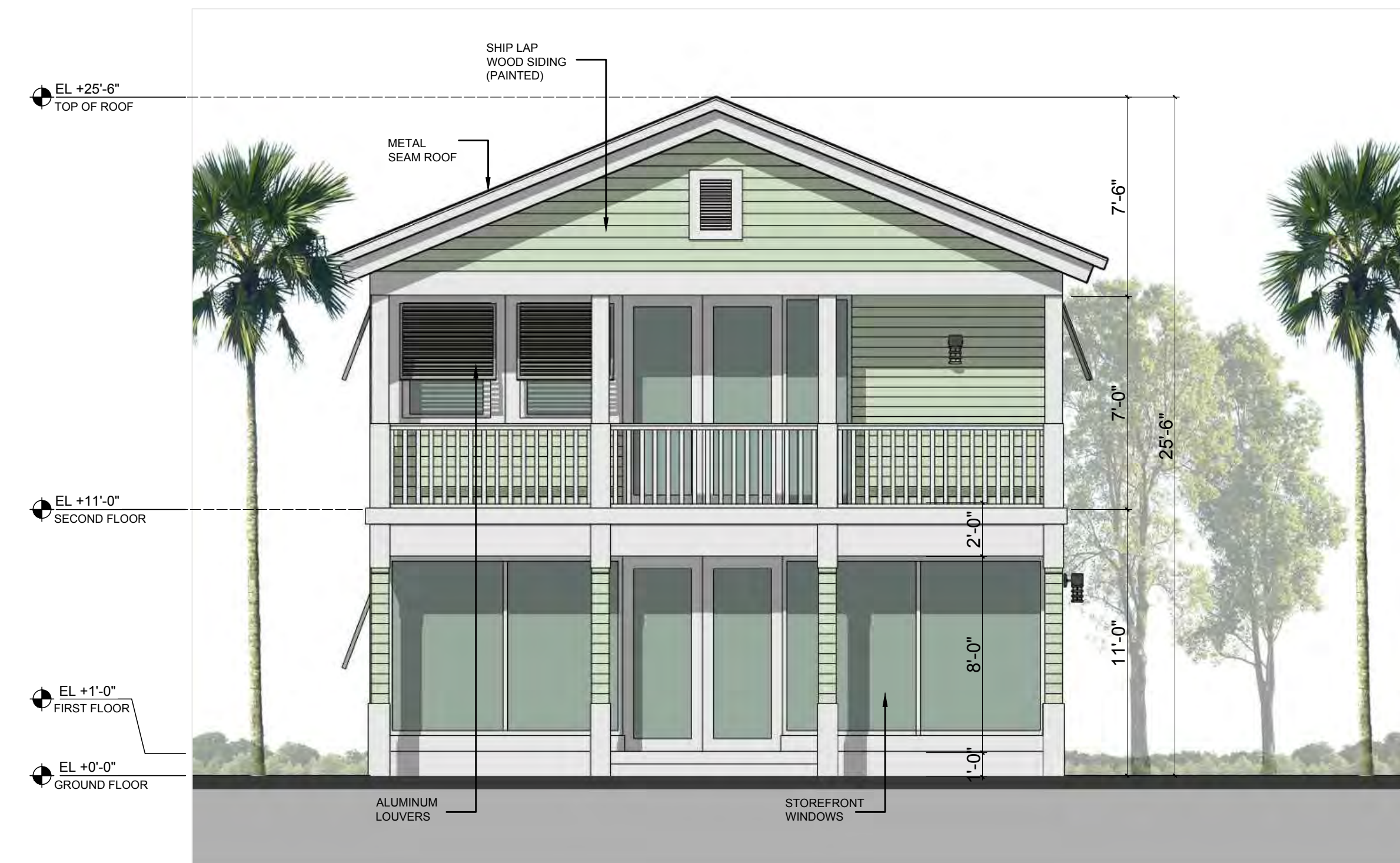
SOUTH-EAST ELEVATION (FRONT)
