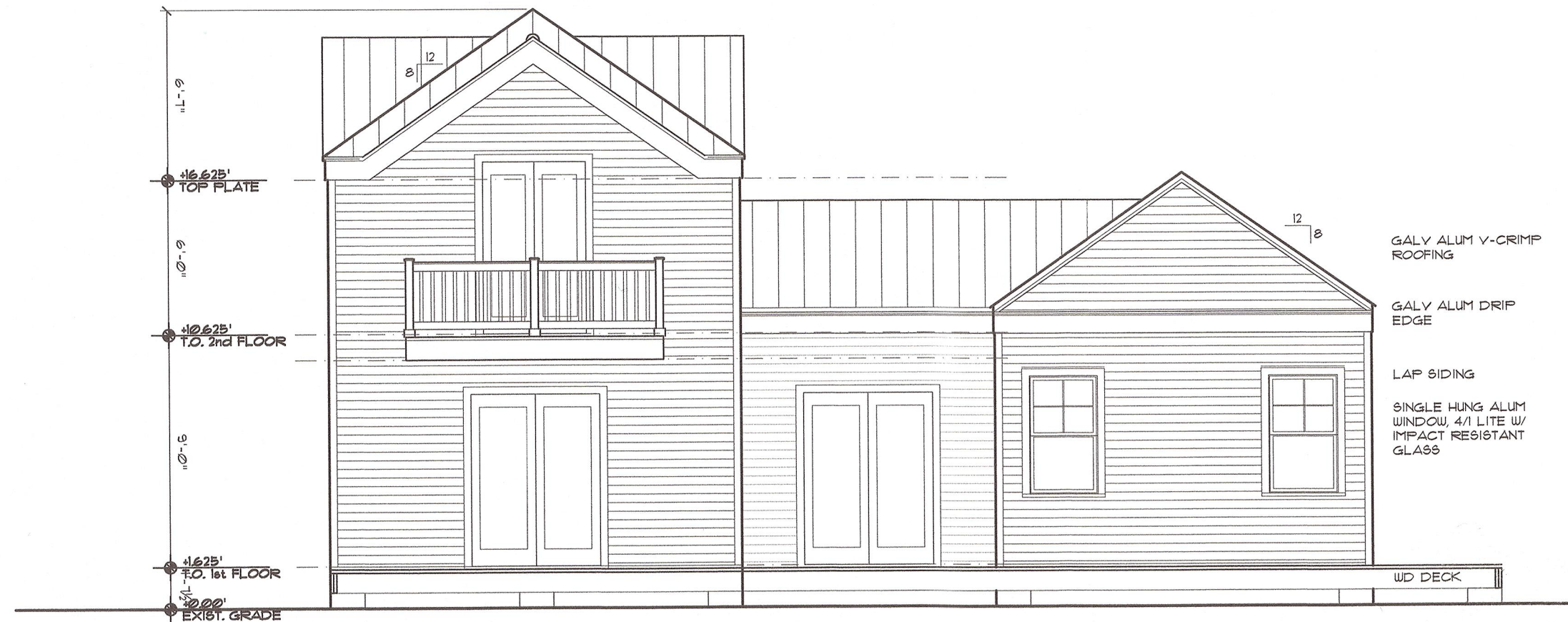
Rear Cottage Front Elevation
