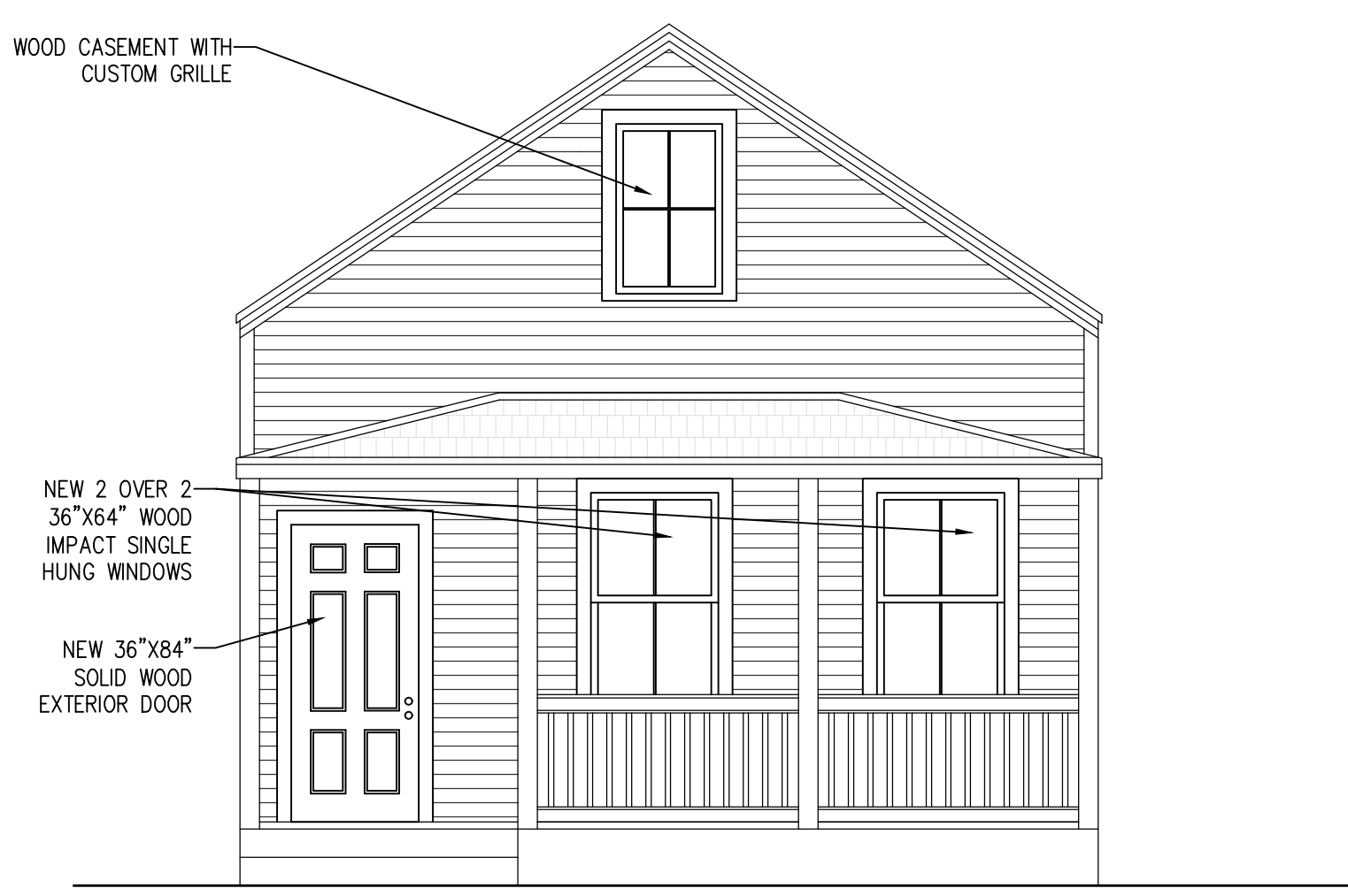
4 PROPOSED FRONT ELEVATION A-3 SCALE: 1/4"=1'-0"
