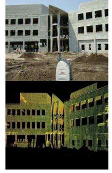
The ScanStation can take a virtual, detailed snapshot of a site including ceilings, undersides of bridges, elevated pipe racks, tall facades, columns and towers. Areas that were previously difficult to access. It collects millions of data points of all items in a 360° horizontal and 270° vertical field of view, allowing a full field of view. This eliminates an additional
