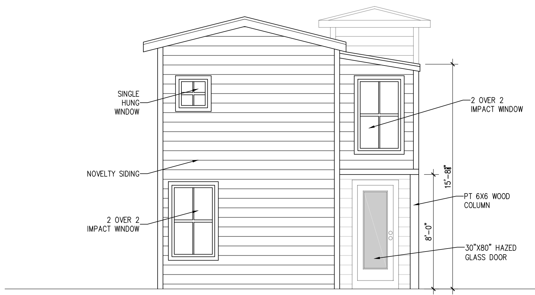
3 PROPOSED FRONT ELEVATION A-2 SCALE: 1/4"=1'-0"
