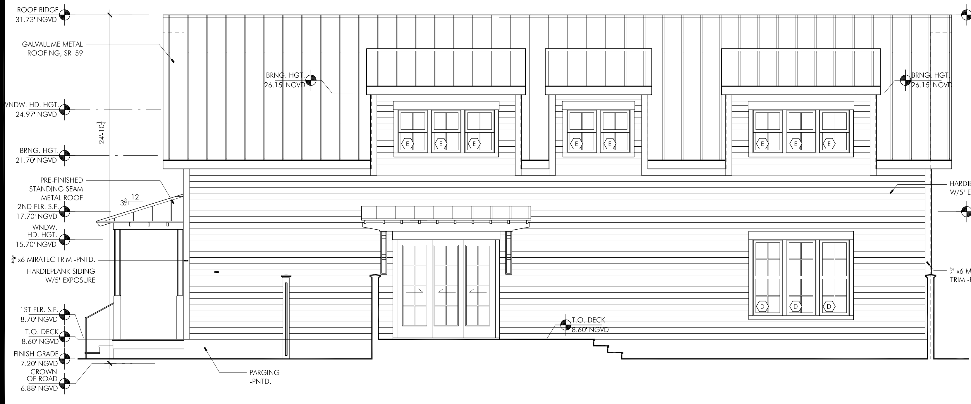
SIDE ELEVATION - UNIT 638 2 1/4" = 1'-0"
