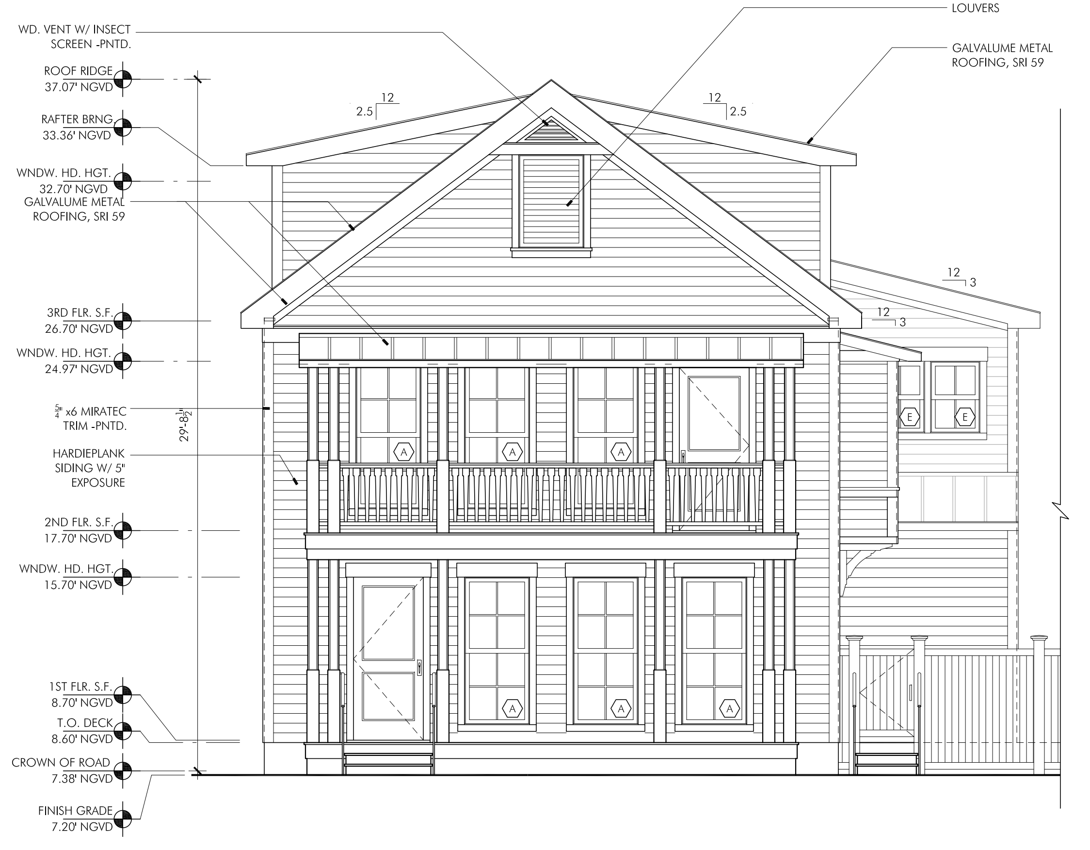
FRONT ELEVATION - UNIT 644 1 1/4" = 1'-0"
