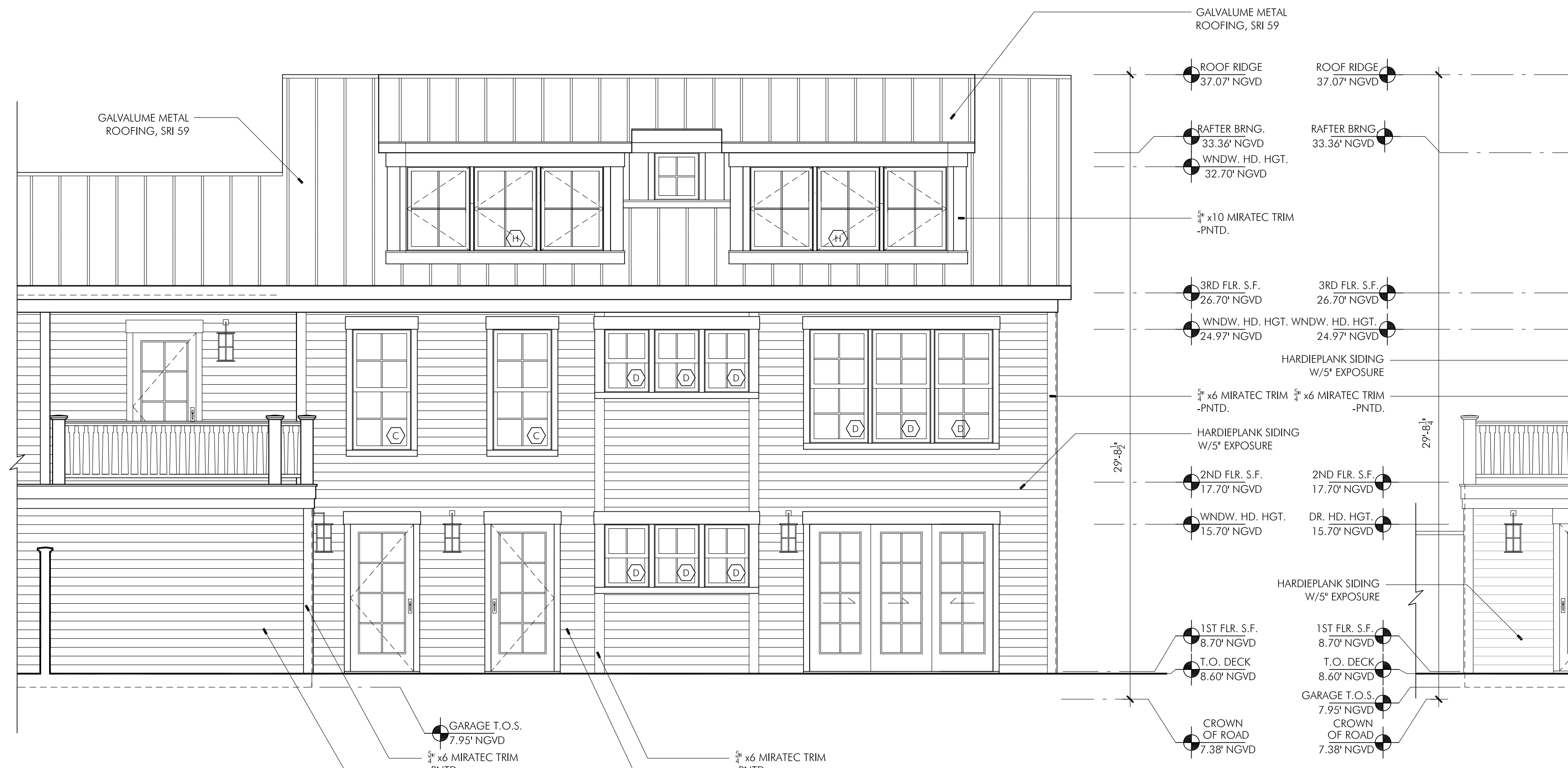
SIDE ELEVATION - UNIT 640 4 1/4" = 1'-0"
