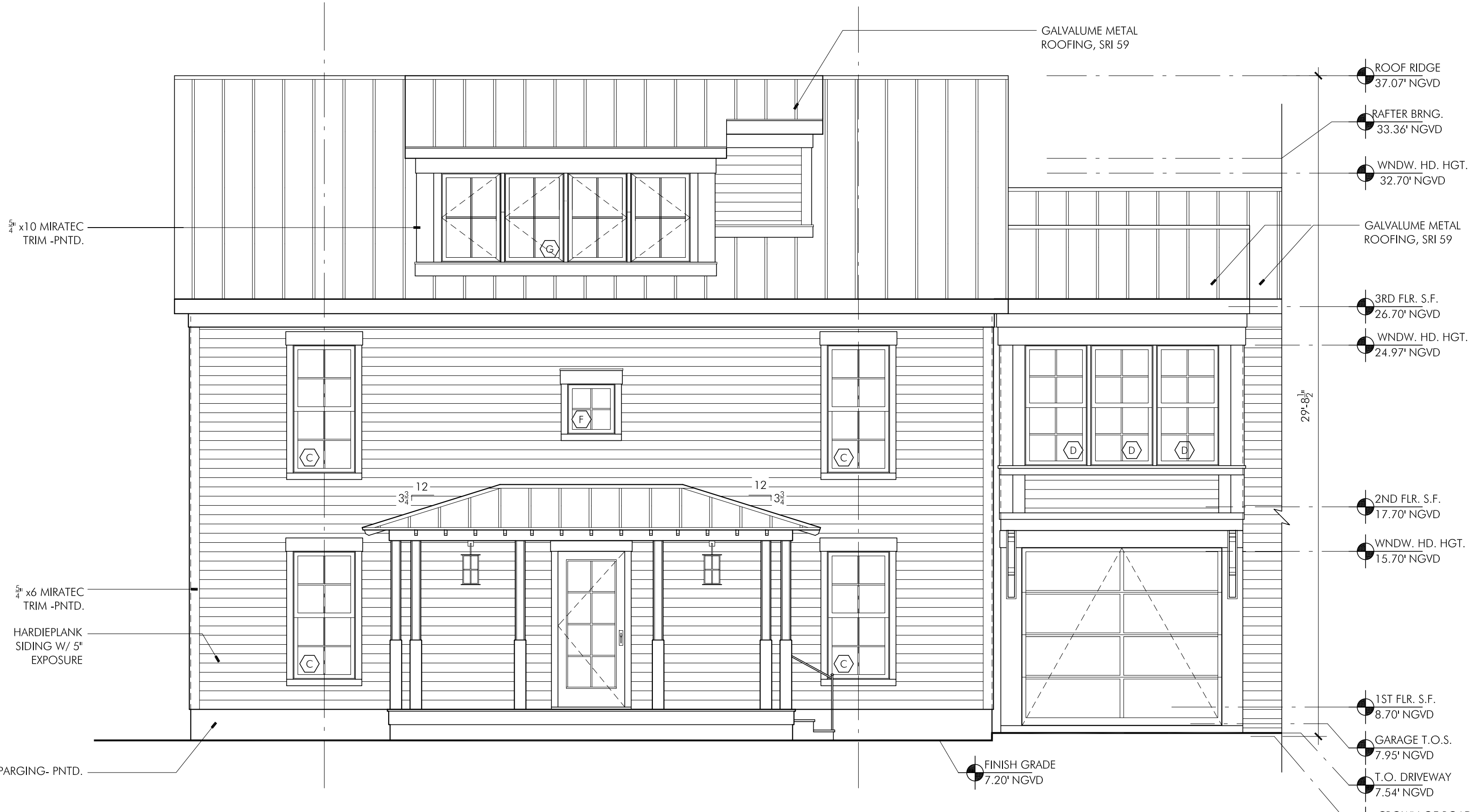
SIDE ELEVATION - UNIT 640 2 1/4" = 1'-0"
