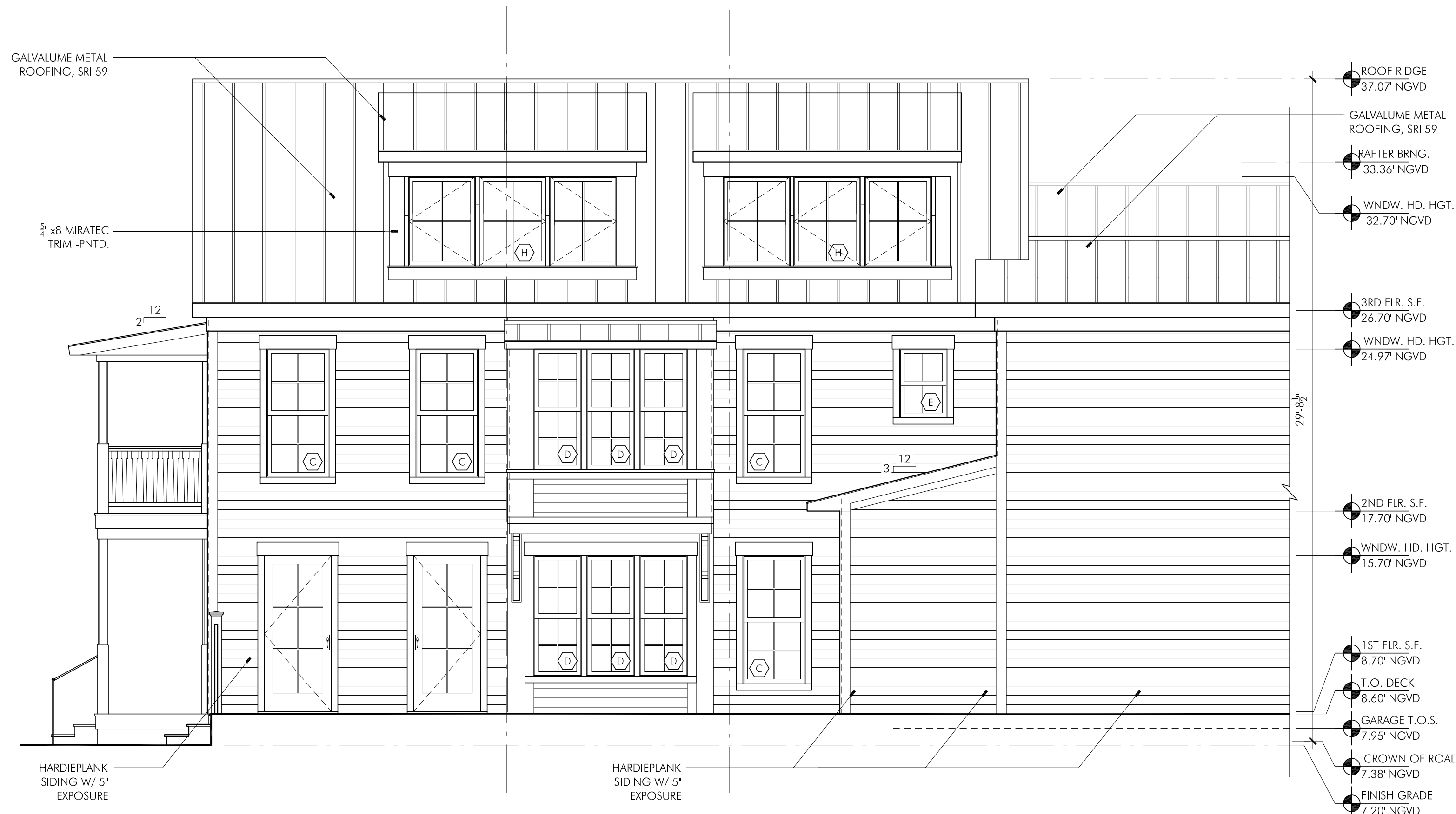
SIDE ELEVATION - UNIT 644 4 1/4" = 1'-0"
