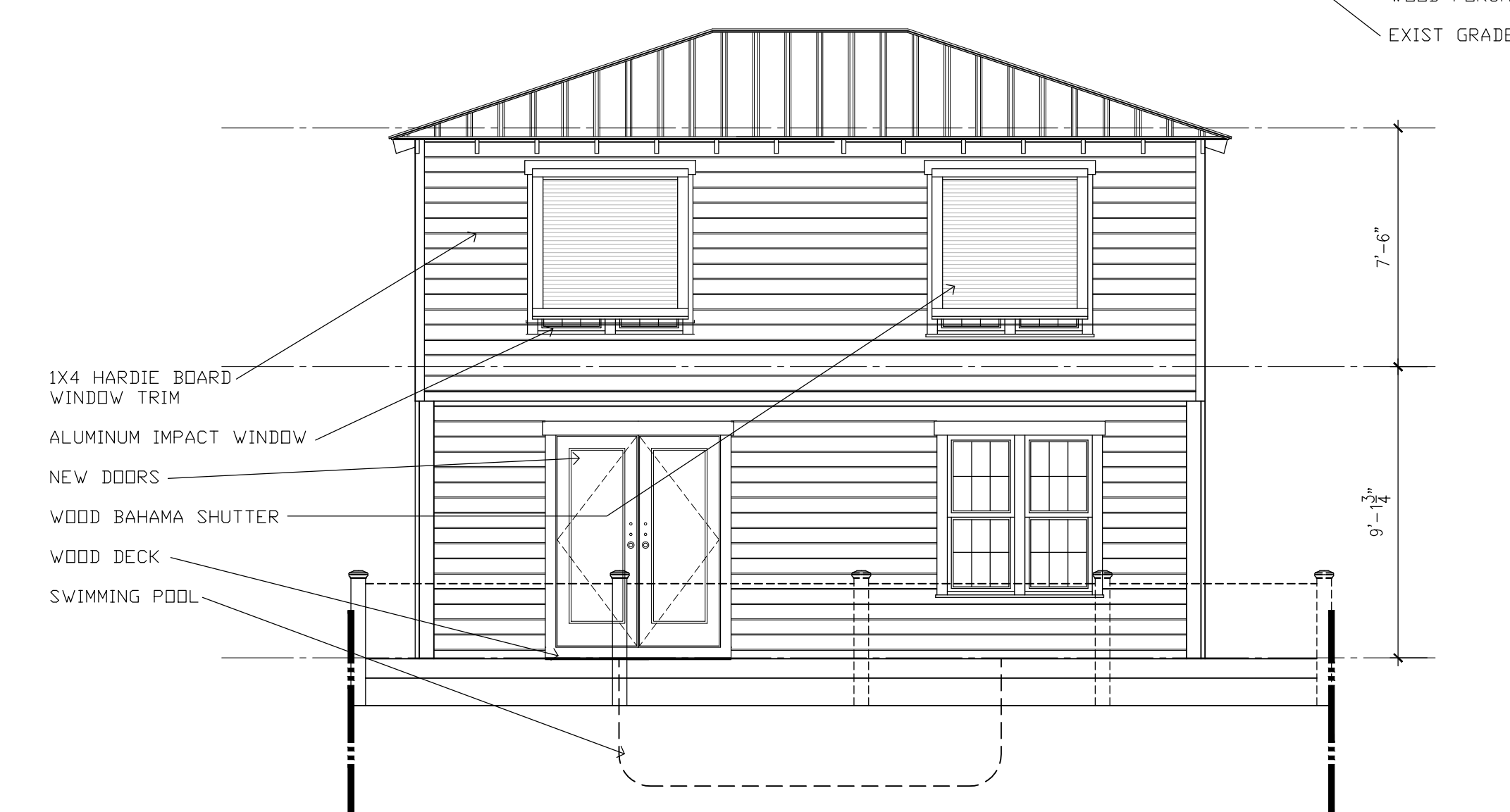
1 PROPOSED FRONT ELEVATION A-2.1 SCALE: 1/4"=1'-0"
