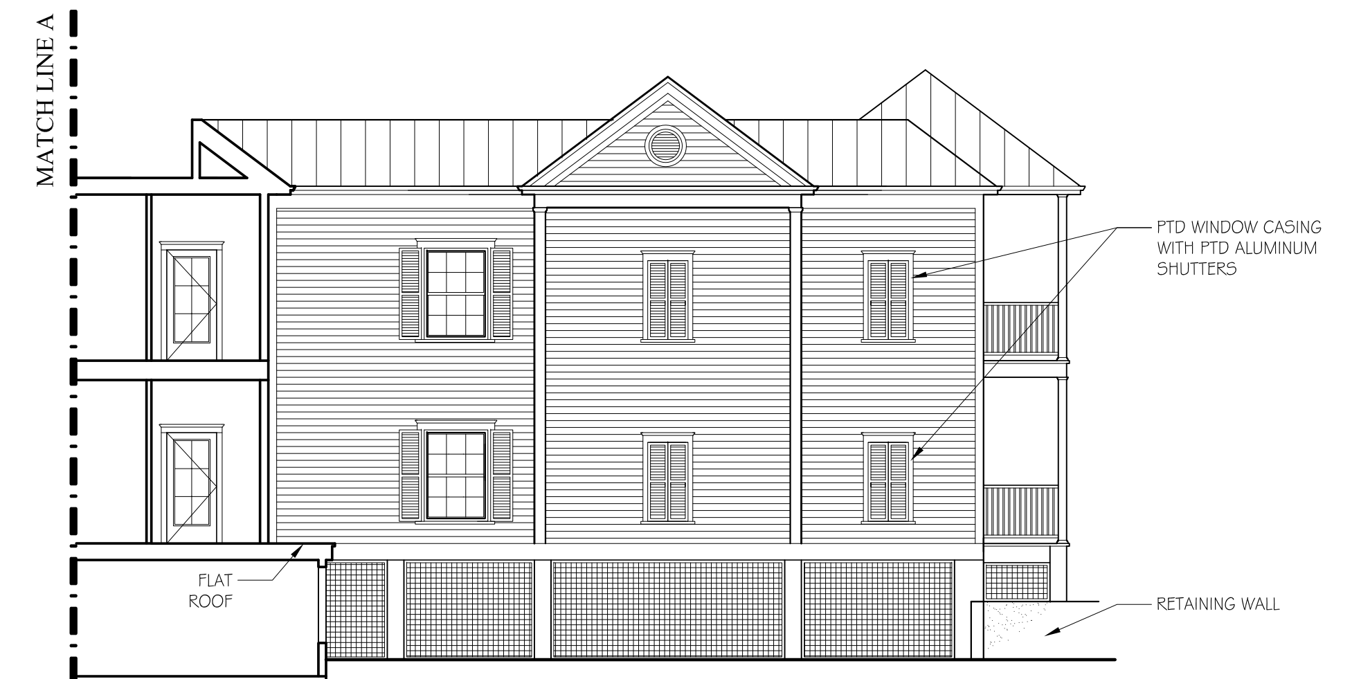
① SOUTH COURTYARD ELEVATION/SECTION SCALE: 1/8"=1'-0"
