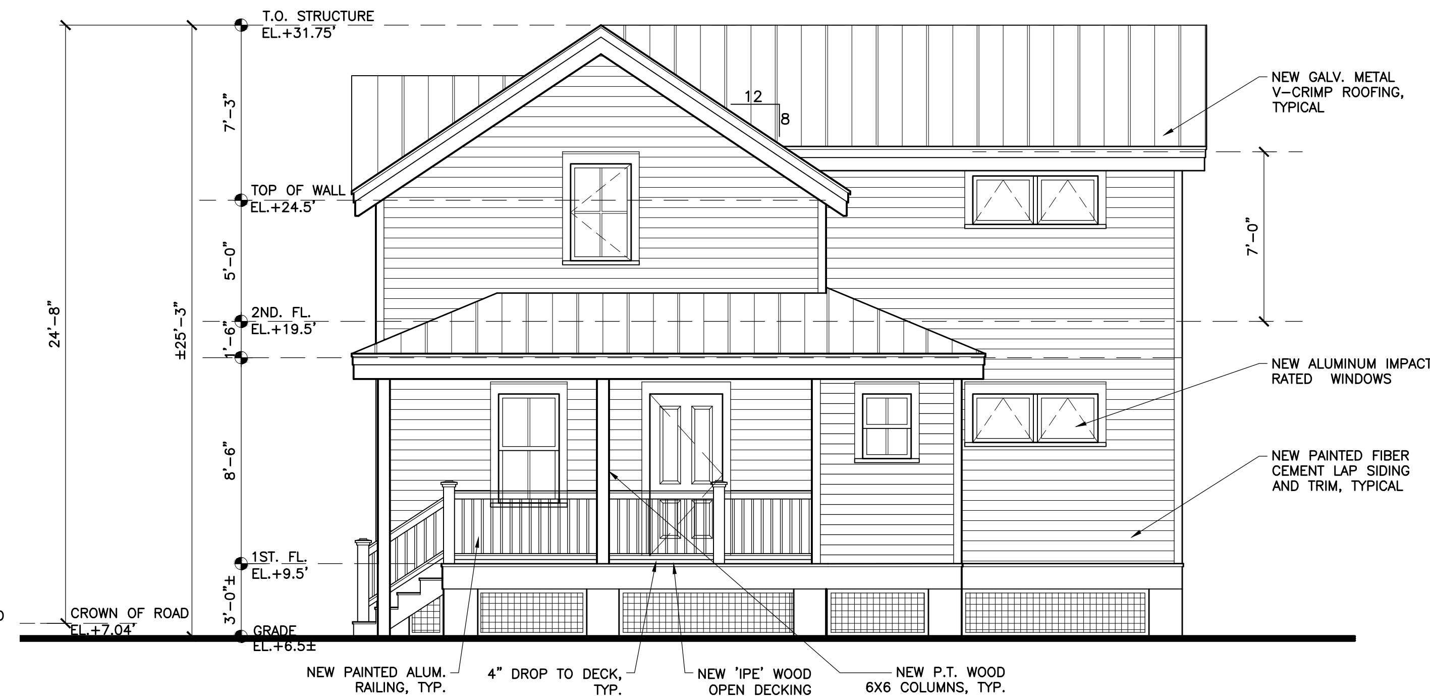
2 UNIT 2- NORTHEAST ELEVATION
