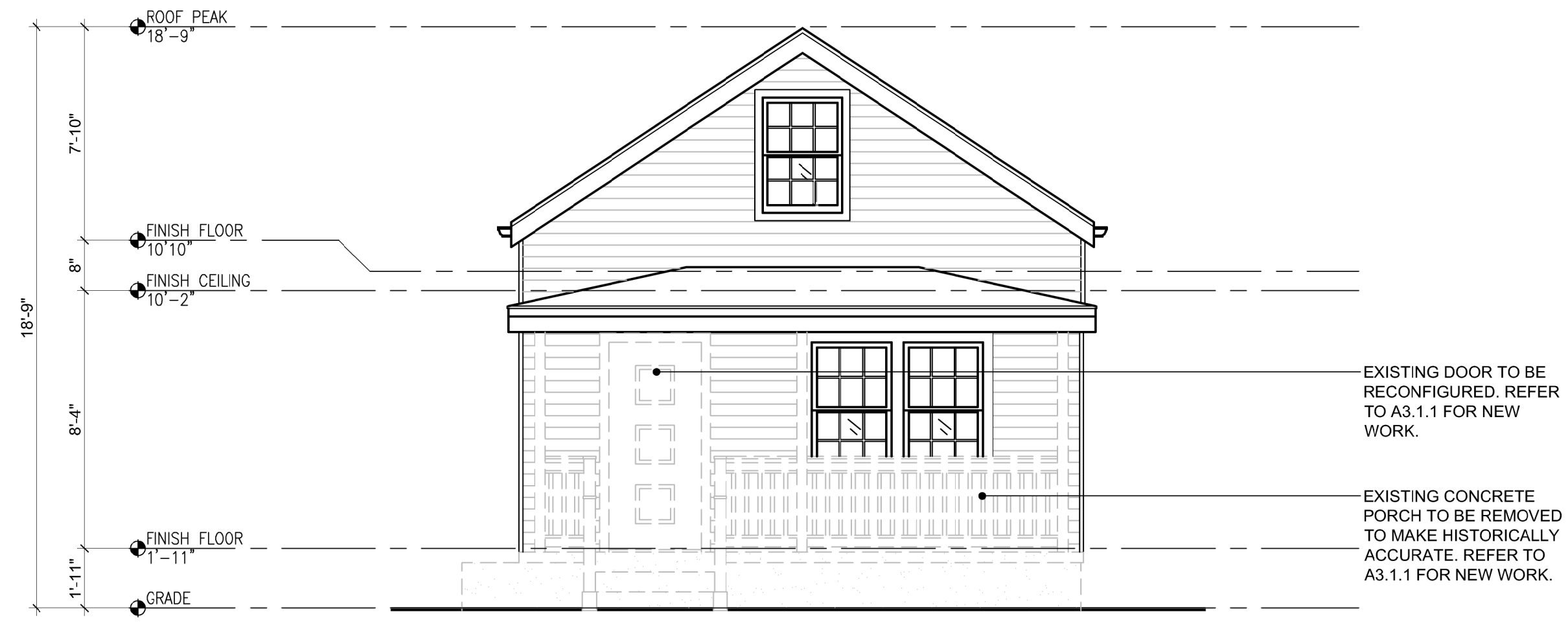
DEMOLITION FRONT ELEVATION SOUTH FACADE
