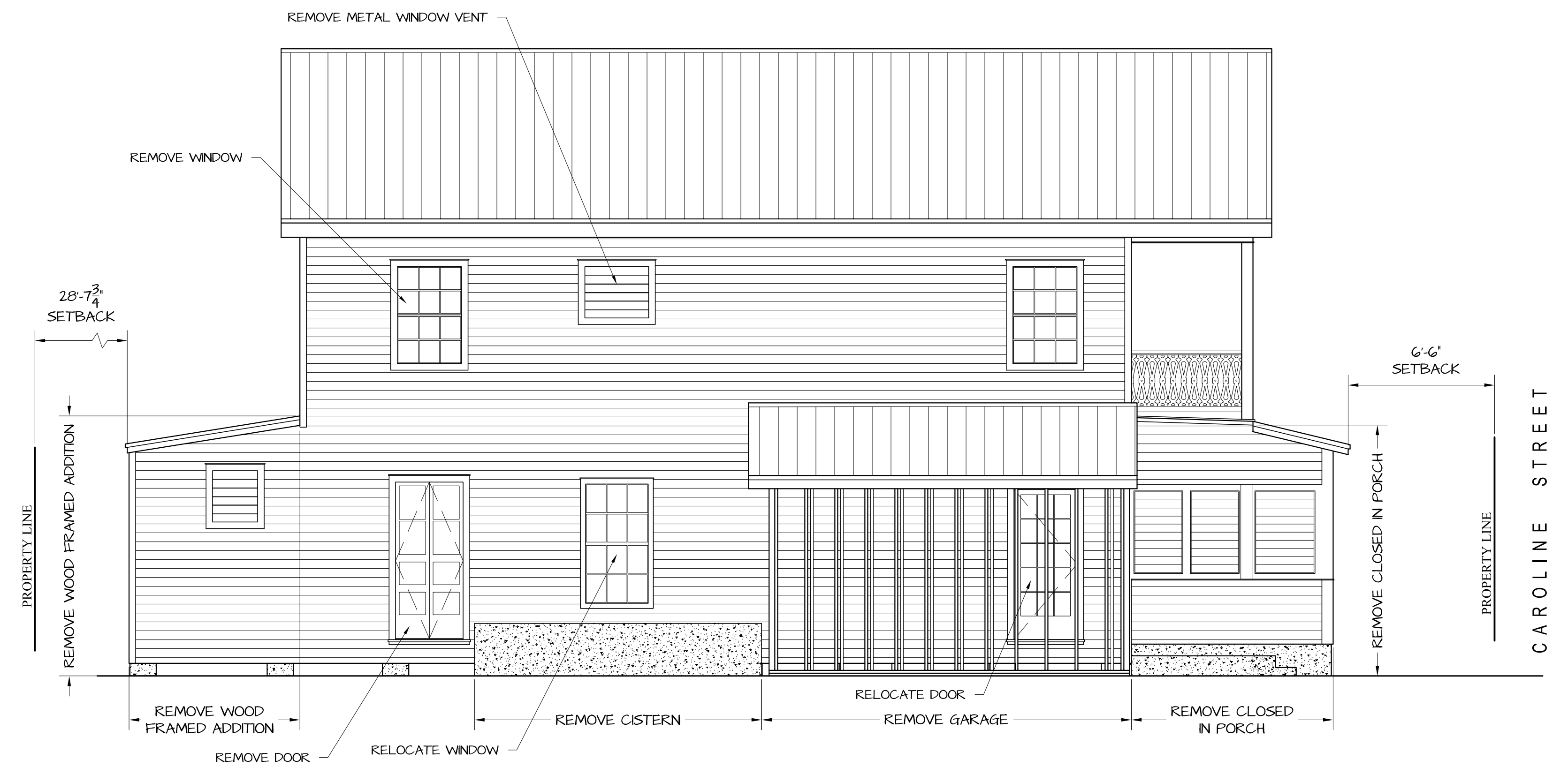
WEST ELEVATION (EXISTING/ DEMO) 1/4" = 1'-0"
