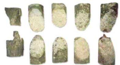
Day 0 | Day 1 | Day 7 | Day 14 | Day 28 Cylinders of common pipe rehab OPC product shear on the cold joint in all cases tested.
