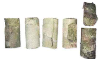
Day 0 | Day 1 | Day 7 | Day 14 | Day 28 GeoSpray geopolymer slant shear cylinders tested in compression don't have cold joints.
