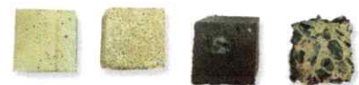
Day 0 | Day 81 | Day 0 | Day 81 OPC loses 50% of its mass when exposed to 7% sulfuric acid; geopolymer mortar is an order of magnitude better in performance.
