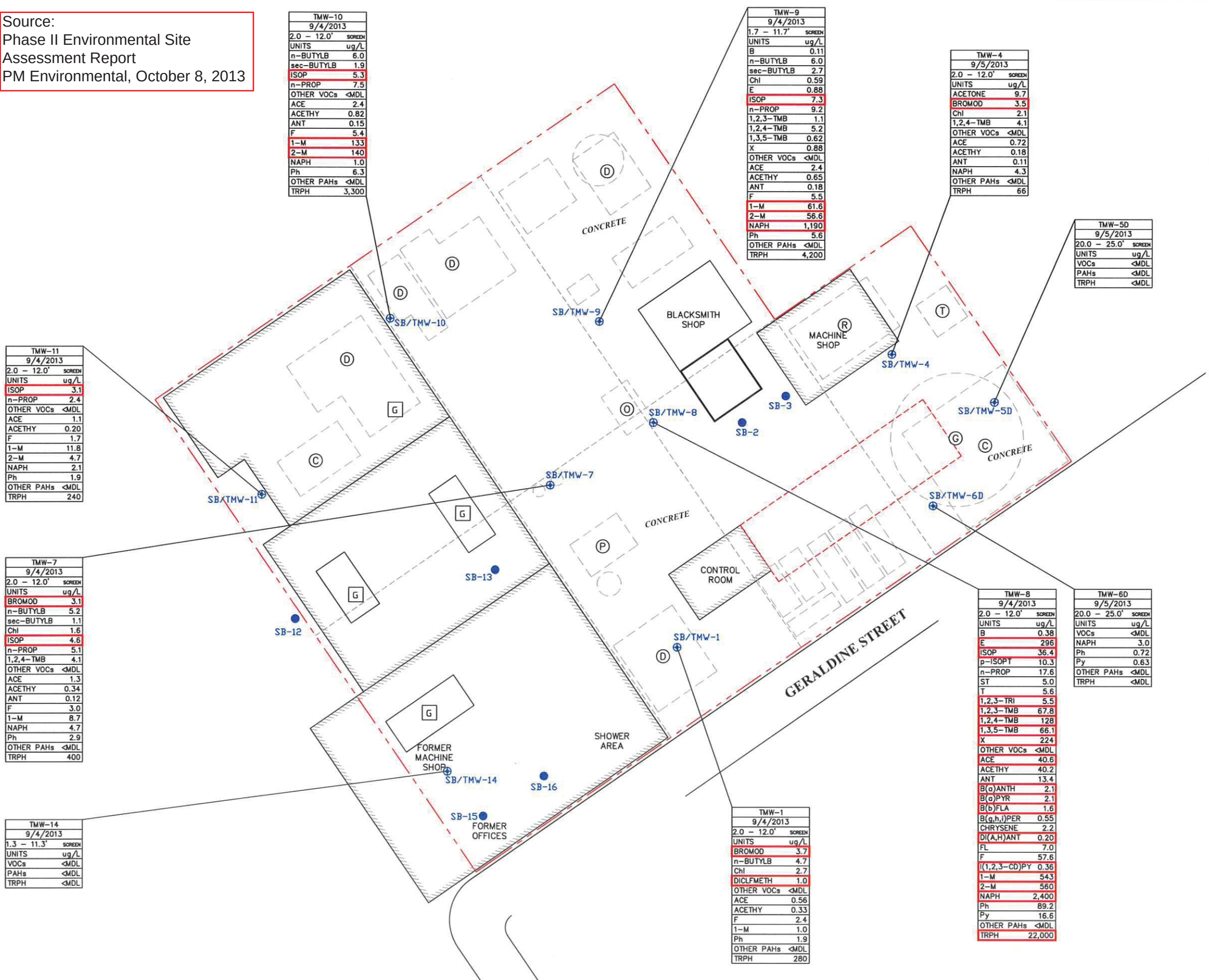
FIGURE 4 SOIL BORING / TEMPORARY MONITORING WELL LOCATION MAP WITH GROUNDWATER ANALYTICAL RESULTS PROJ: FORMER KEY WEST GAS AND ELECTRIC COMPANY 101-111 GERALDINE STREET KEY WEST, FL
