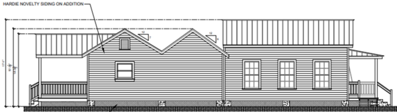
4 PROPOSED SIDE ELEVATION NORTH A-5 SCALE: 1/4" = 1'
