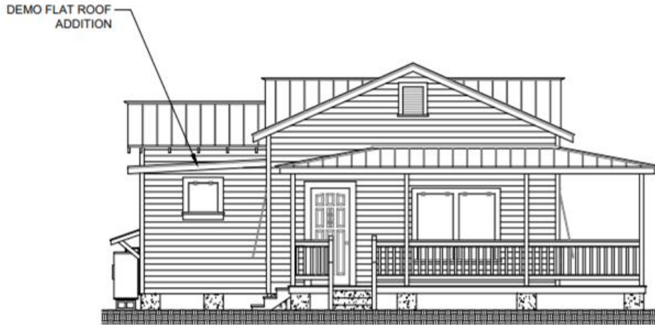
1 A-4 EXISTING FRONT ELEVATION WEST SCALE: 1/4" = 1'
