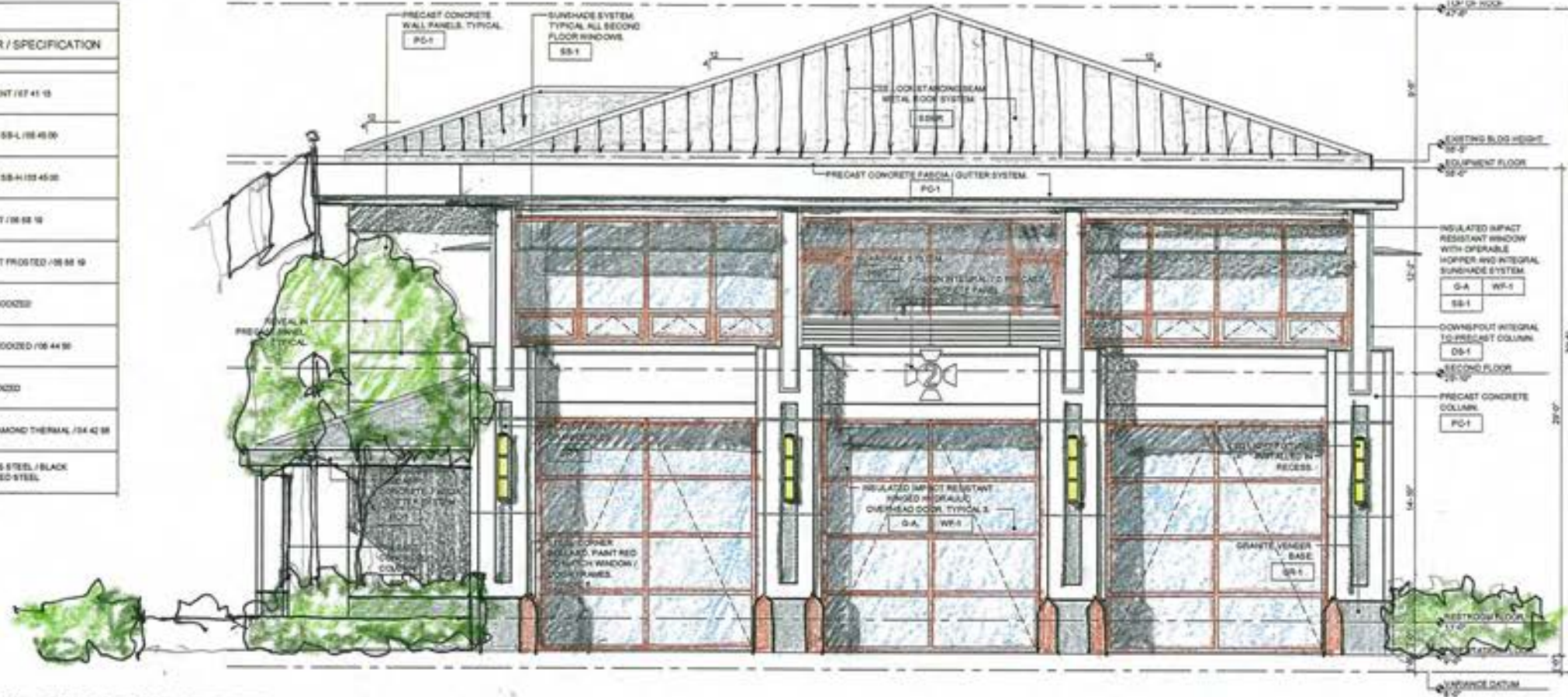
02 EAST ELEVATION - SIMONTON STREET A3.1.1 SCALE: 1/4" = 1'-0"
