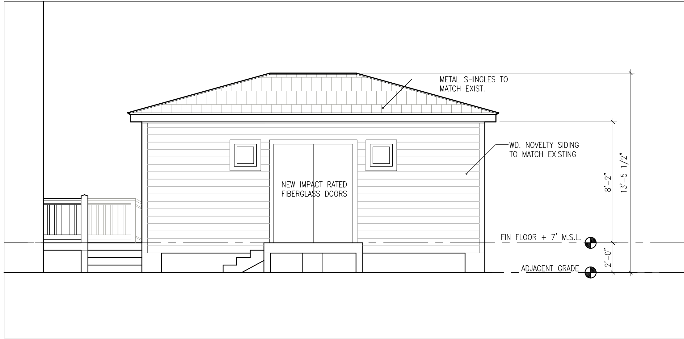
2 A2.1 PROPOSED NORTH ELEVATION SCALE: 1/4"=1'-0"
