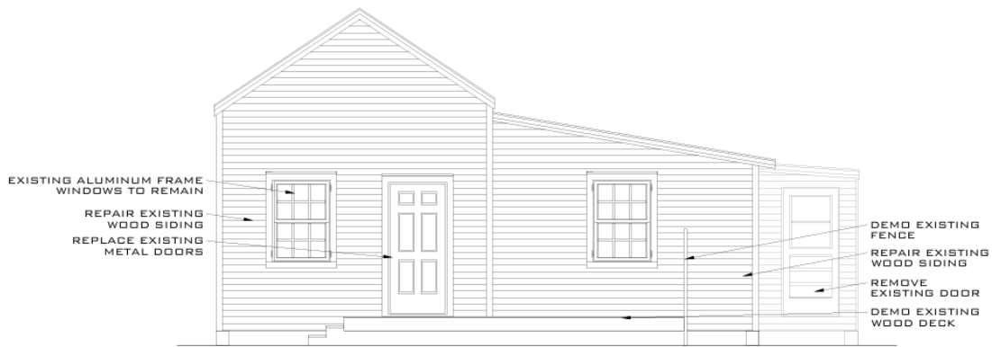
EXISTING FRONT ELEVATION
