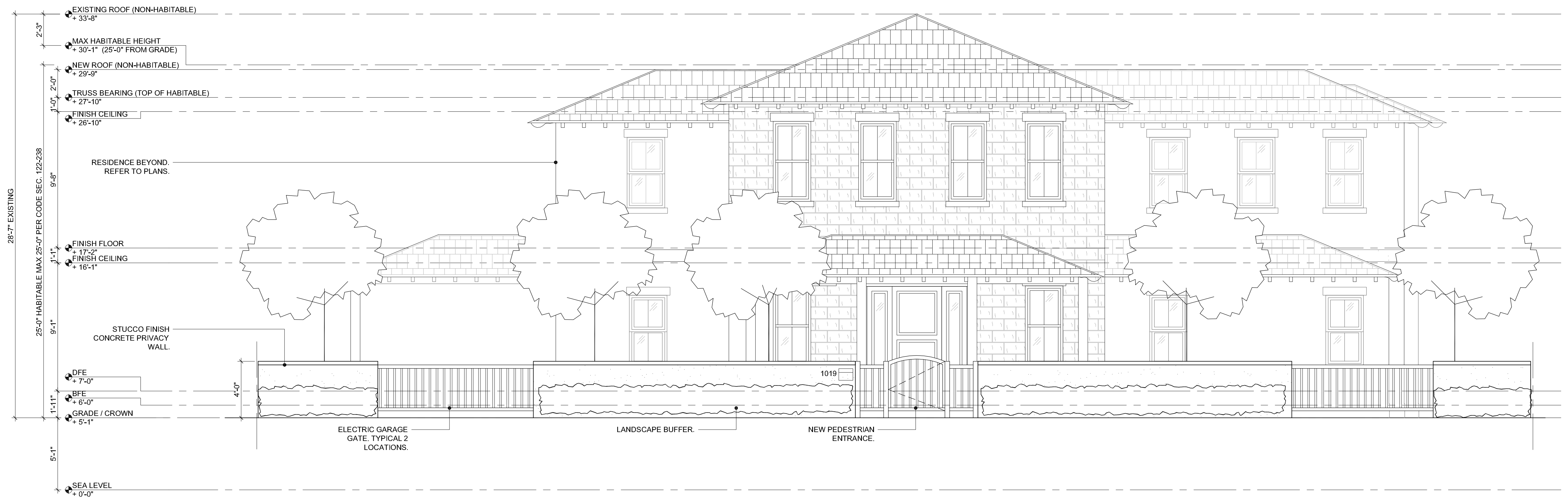
1 A3.1.3 SOUTH ELEVATION - STREET VIEW SCALE: 1/4" = 1'-0"
