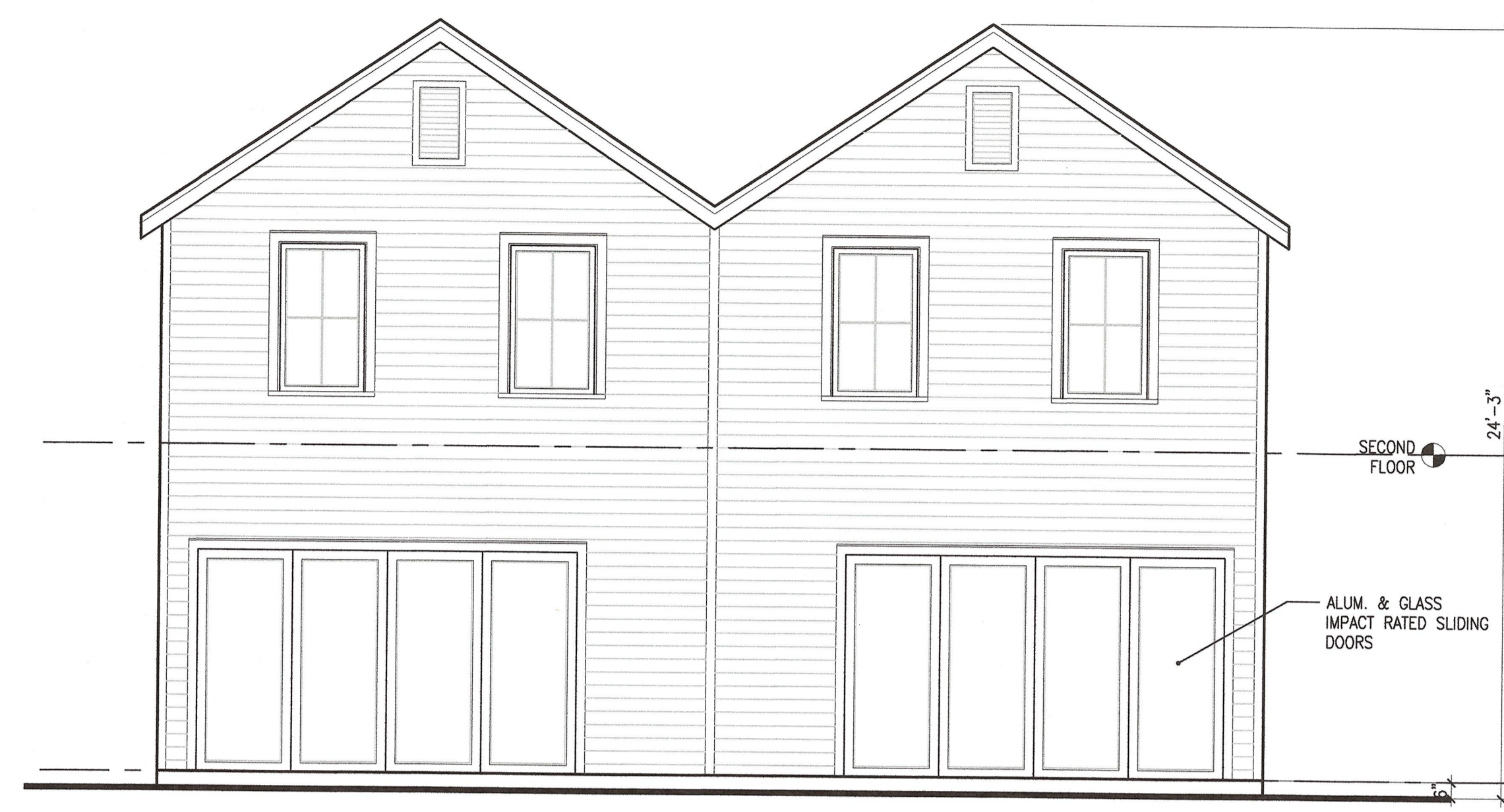
3 RESIDENTIAL SOUTH ELEVATION SCALE: 1/4"=1'-0" A3.2
