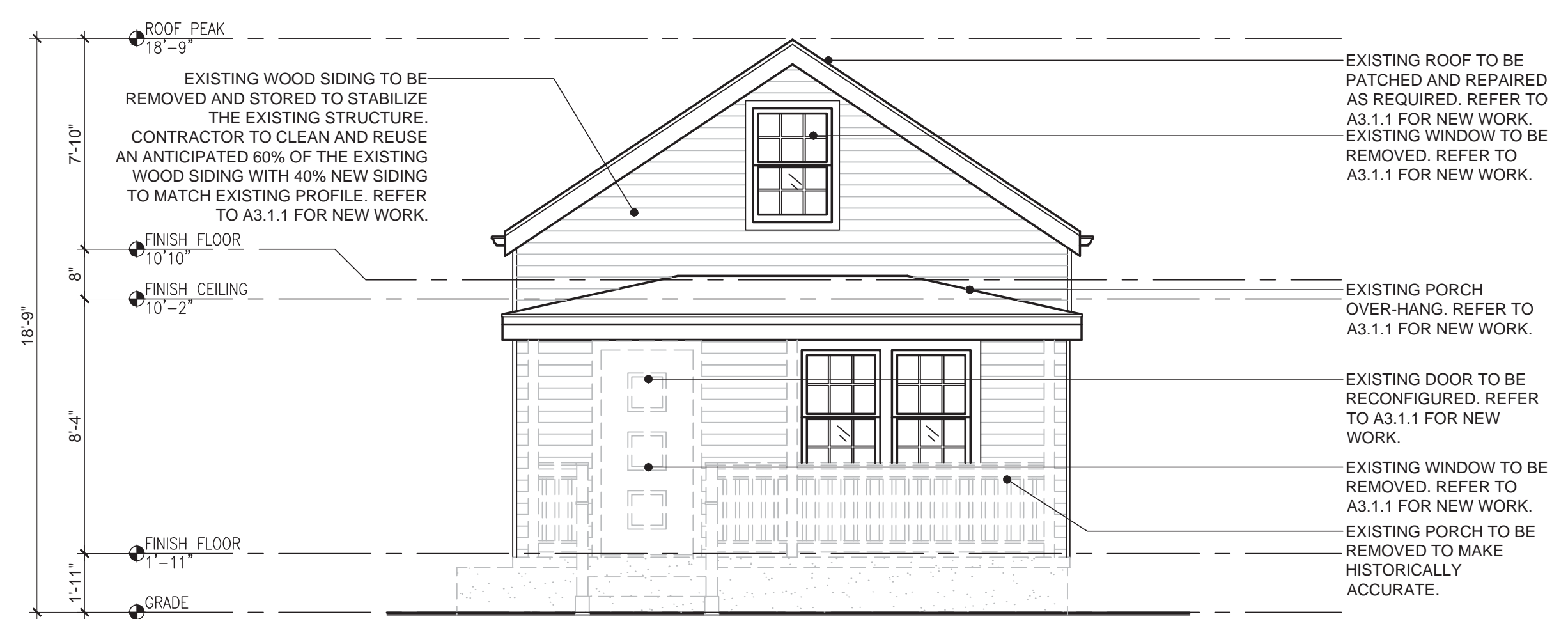
1 DEMOLITION SOUTH ELEVATION SCALE: 1/4"=1'-0"
