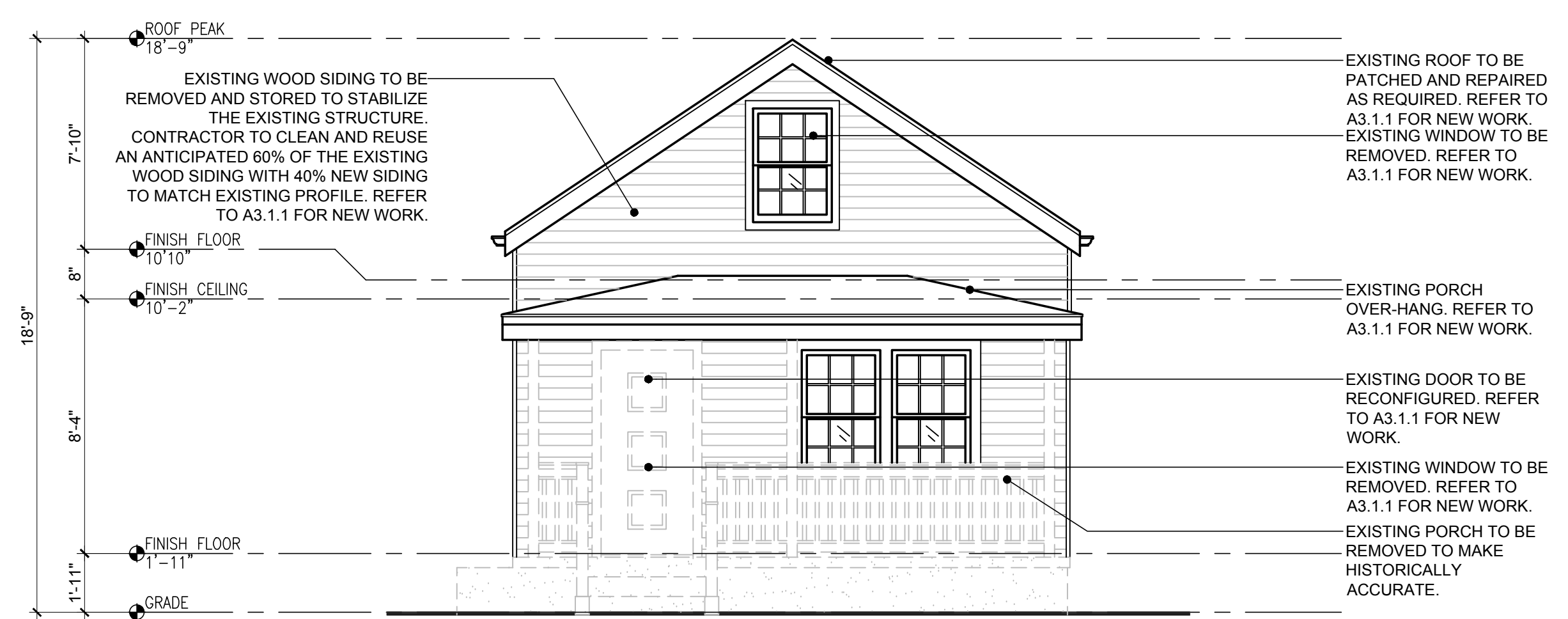
1 DEMOLITION SOUTH ELEVATION SCALE: 1/4"=1'-0"
