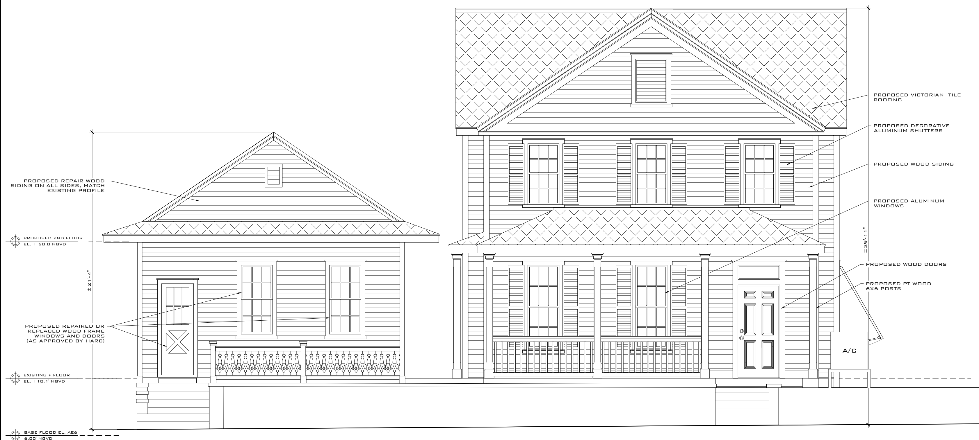
PROPOSED FRONT ELEVATION SCALE: 1/4" = 1'-0"
