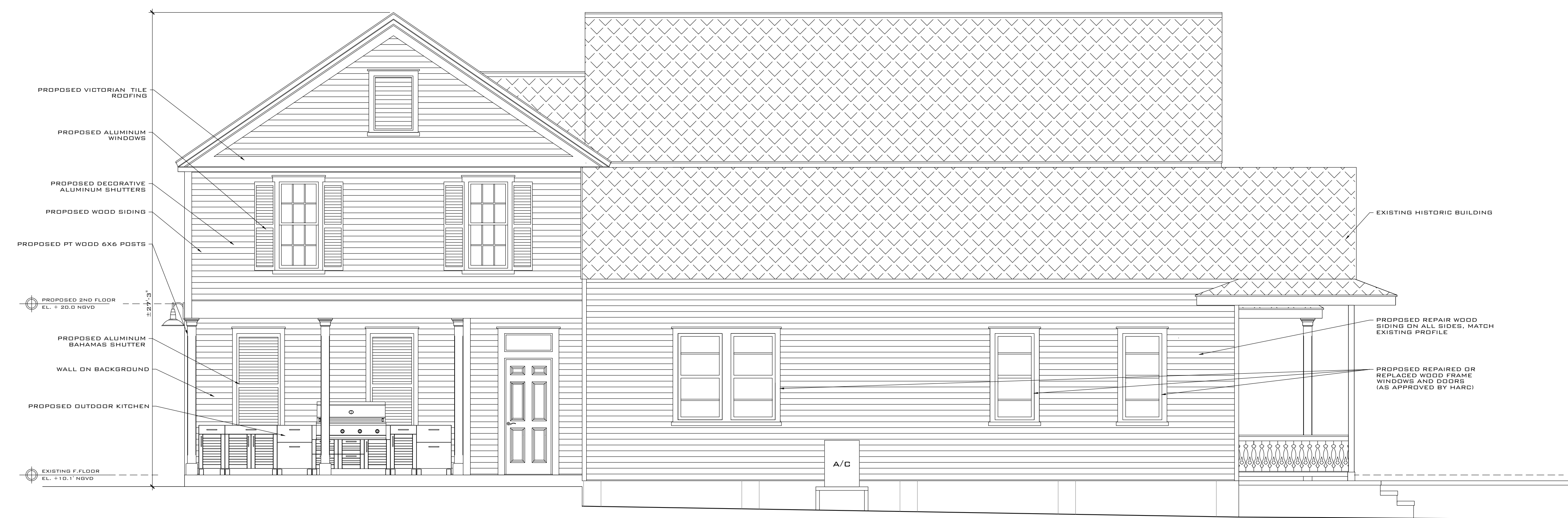
PROPOSED LEFT ELEVATION SCALE: 1/4" = 1'-0"
