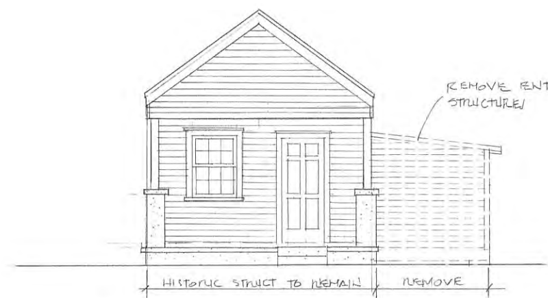
EXISTING / DEMOLITION - FRONT ELEVATION
