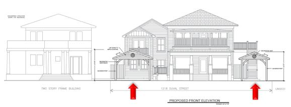
Proposed Front Elevation. Arrows indicate proposed carports, and neighboring structure displays no carport.
