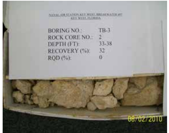
TB-3, Core Run 2, Depth Interval 33-38 feet
