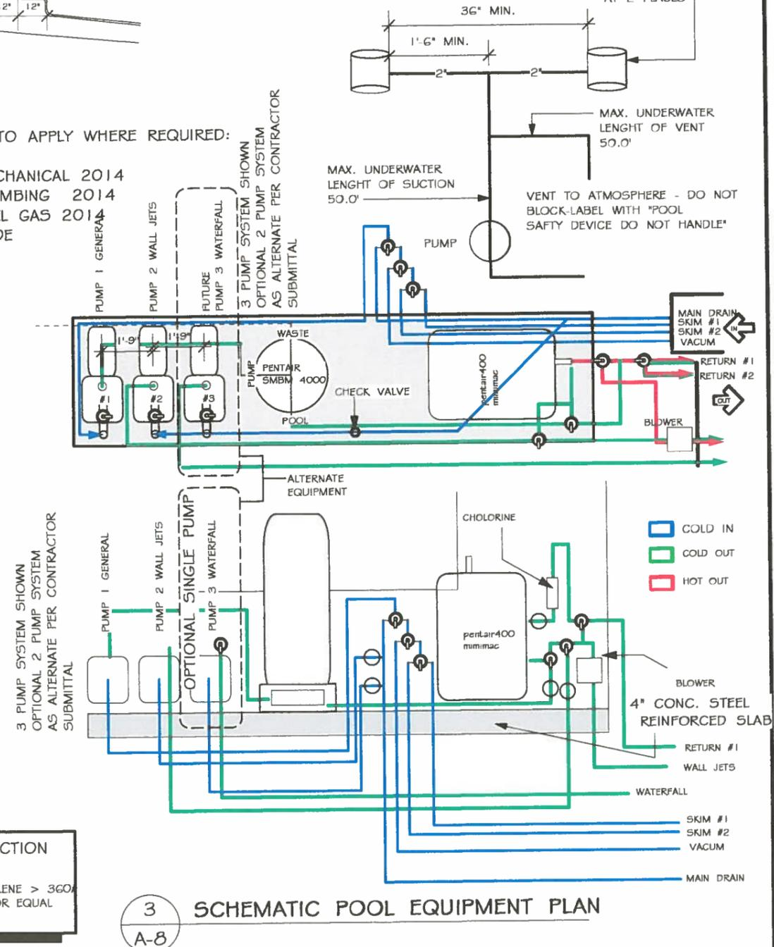
3 SCHEMATIC POOL EQUIPMENT PLAN
