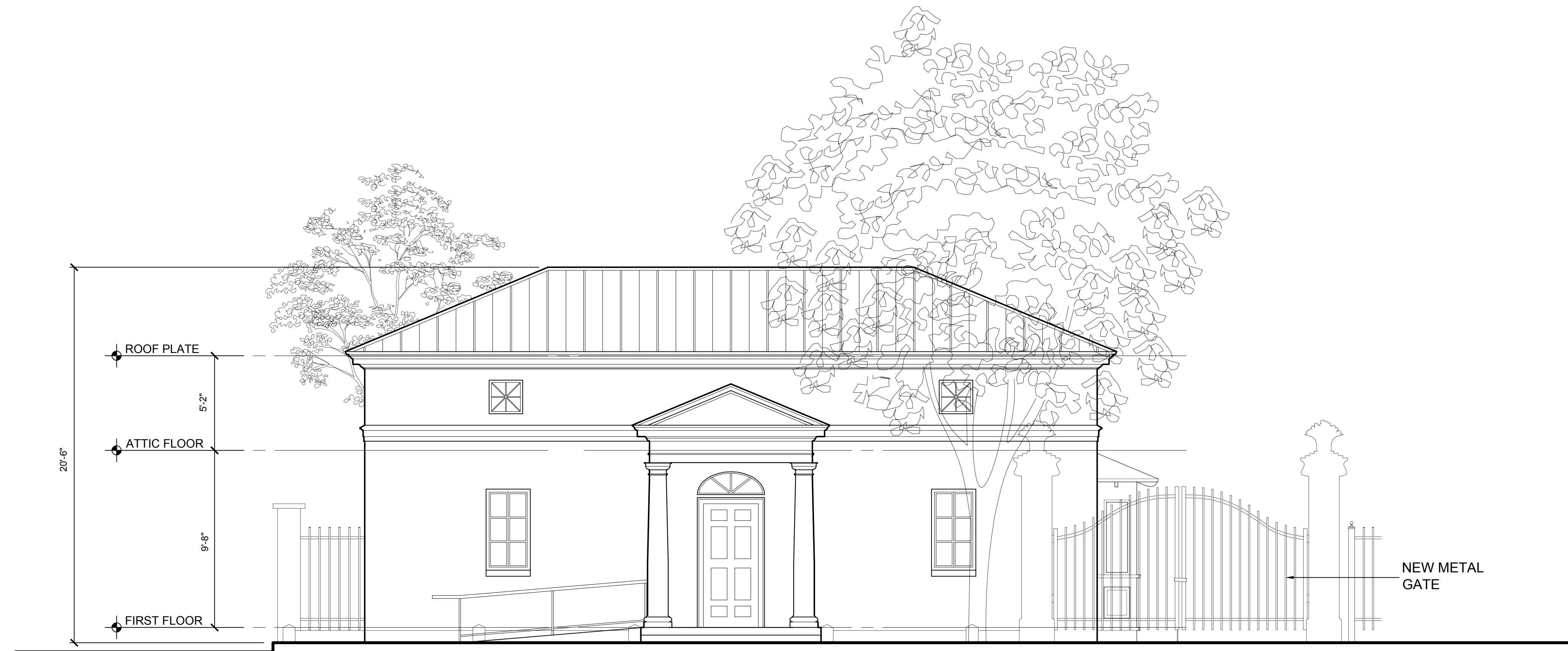
WEST ELEVATION SCALE: 1/4"=1'-0"
