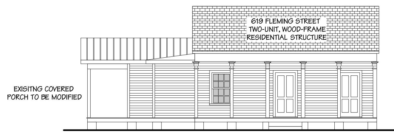
EXISTING FRONT ELEVATION scale: 1/8"=1'-0"
