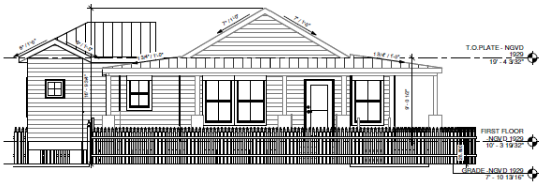
2 FRONT ELEVATION - PROPOSED 1/4" = 1'-0"
