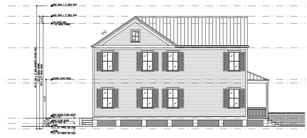
2 PROPOSED SIDE ELEVATION SCALE: 1/4" = 1'-0"
