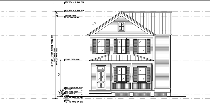
1 PROPOSED FRONT ELEVATION SCALE: 1/4" = 1'-0"
