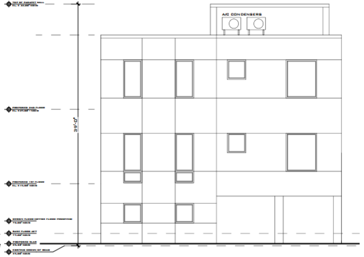
PROPOSED REAR ELEVATION SCALE: 1/8" = 1'-0"
