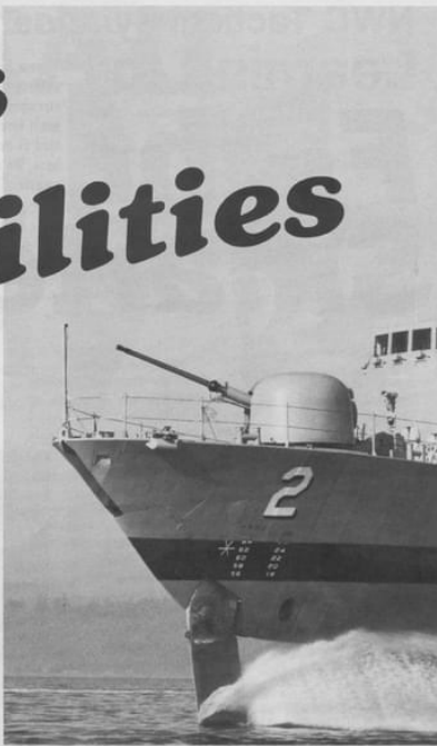
▲ Foilborne configuration of a PHM is demonstrated by USS Hercules (PHM 2) during sea trials. Hercules and USS Gemini (PHM 6) will join PHMRON TWO in Key West later this month.
