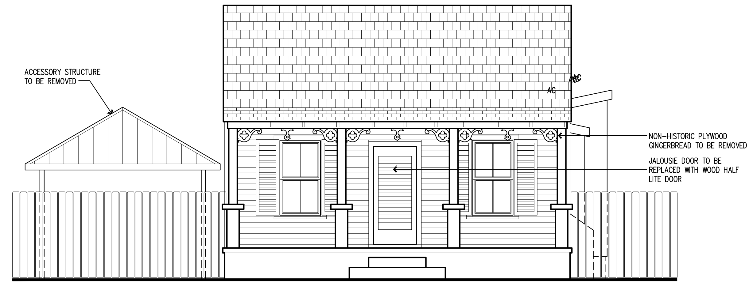
EXISTING FRONT ELEVATION 1/4"=1'-0"
