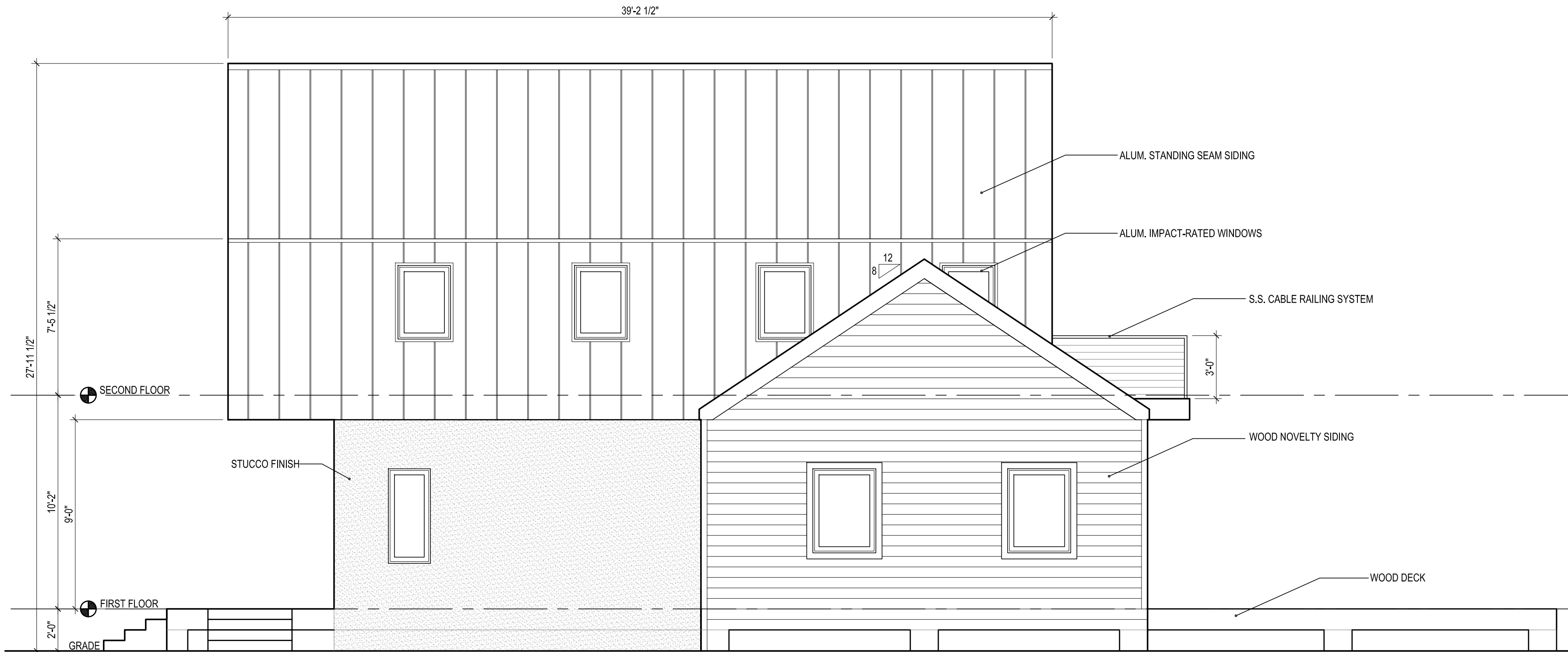
3 A3.1 WEST ELEVATION SCALE: 1/4"=1'-0"
