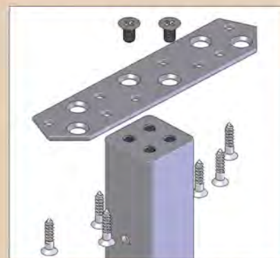
Top Mounting Plate Assembly (fasteners included)
