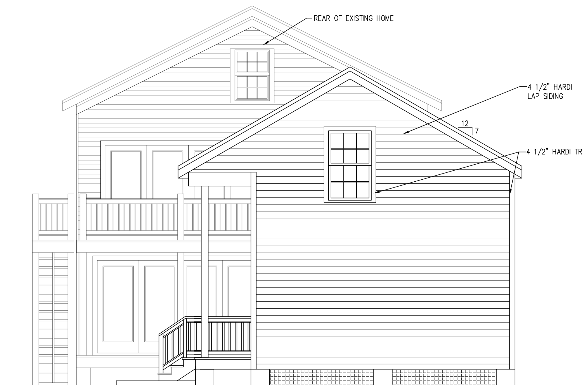
1 A-2 PROPOSED REAR ELEVATION SCALE: 1/4"=1'-0"
