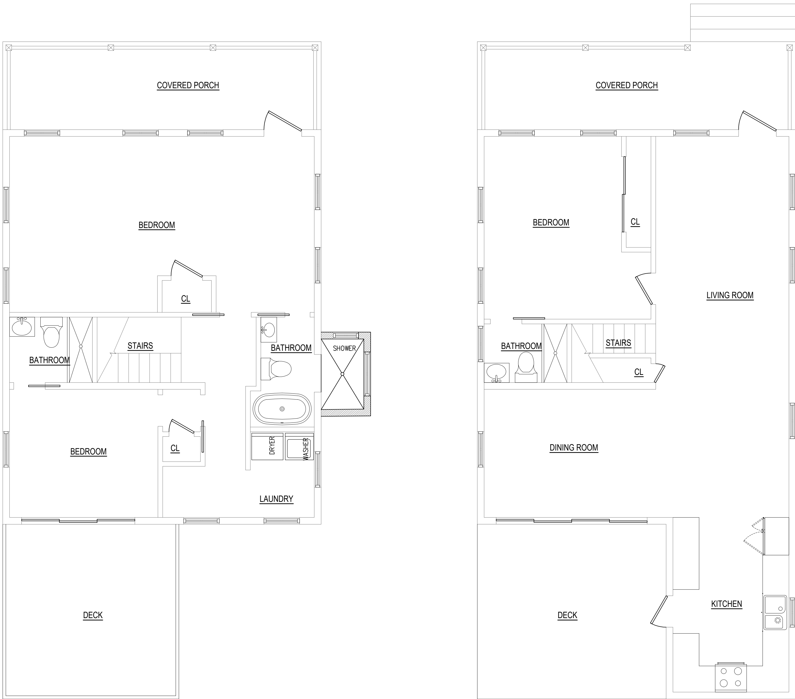
2 "MAIN HOUSE" CURRENT 2ND FLOOR PLAN A-3 SCALE: 1/4"=1'-0"
