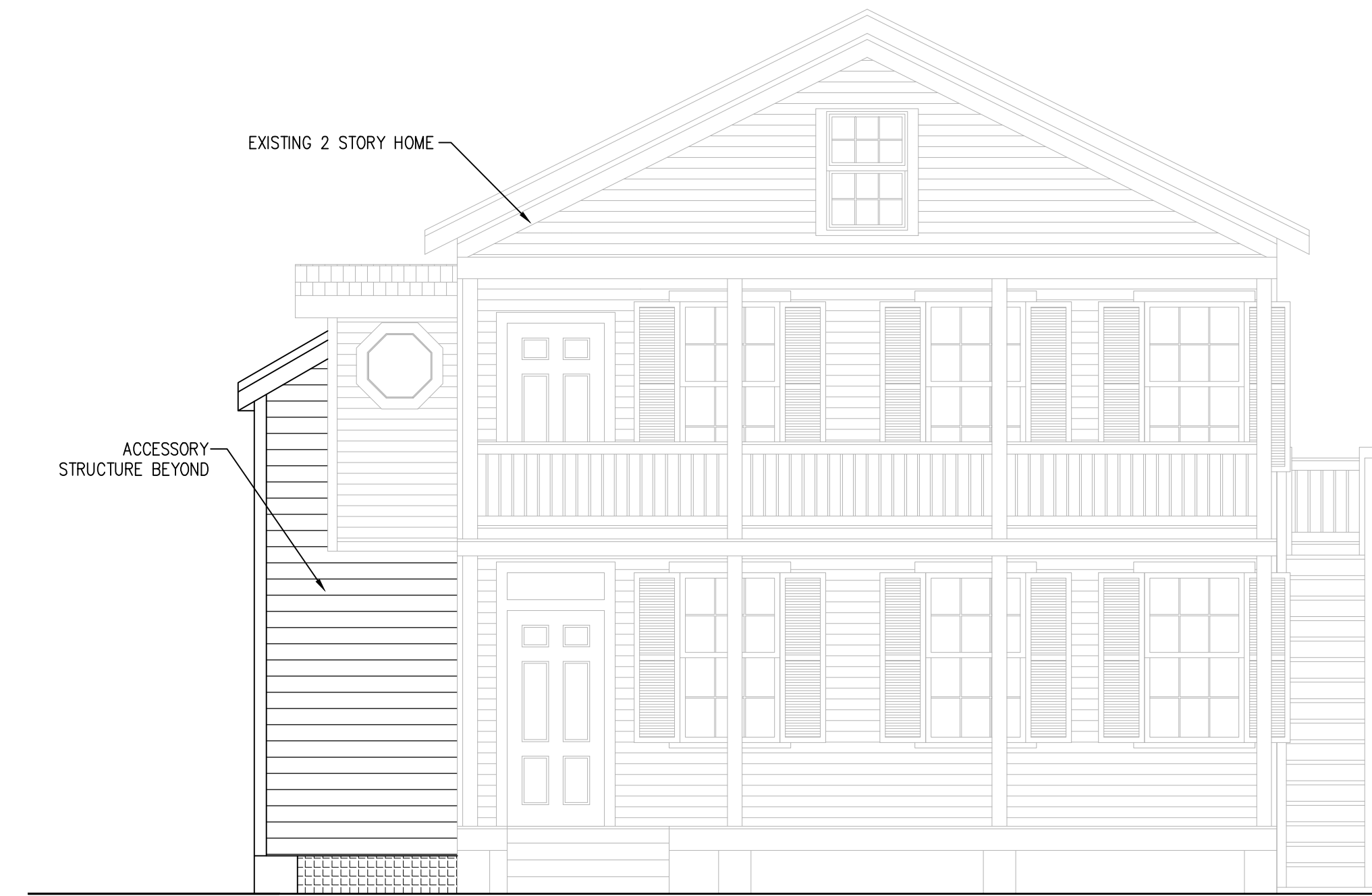
4 A-2 PROPOSED FRONT ELEVATION SCALE: 1/4"=1'-0"
