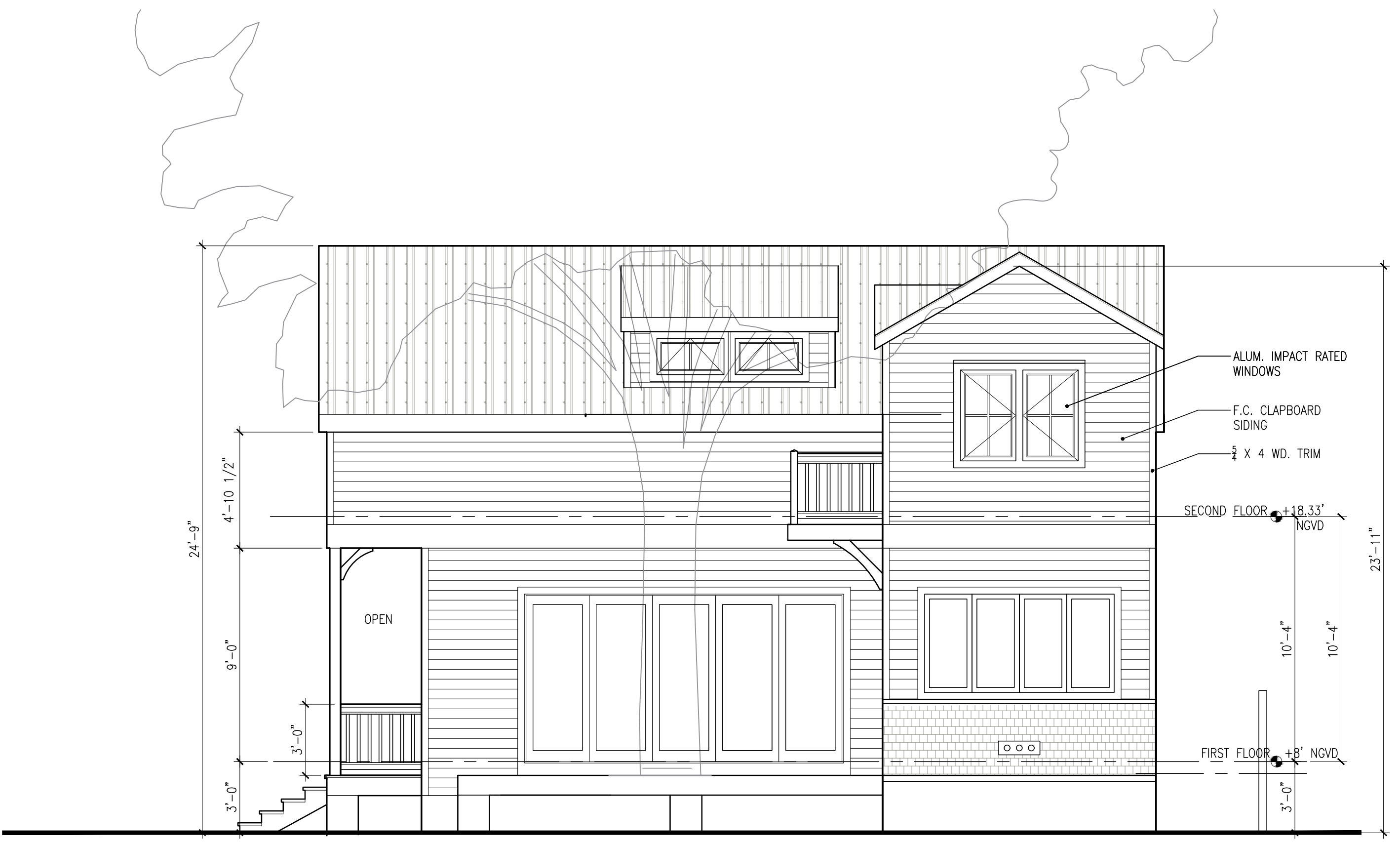
4 EAST ELEVATION SCALE: 1/4"=1'-0"
