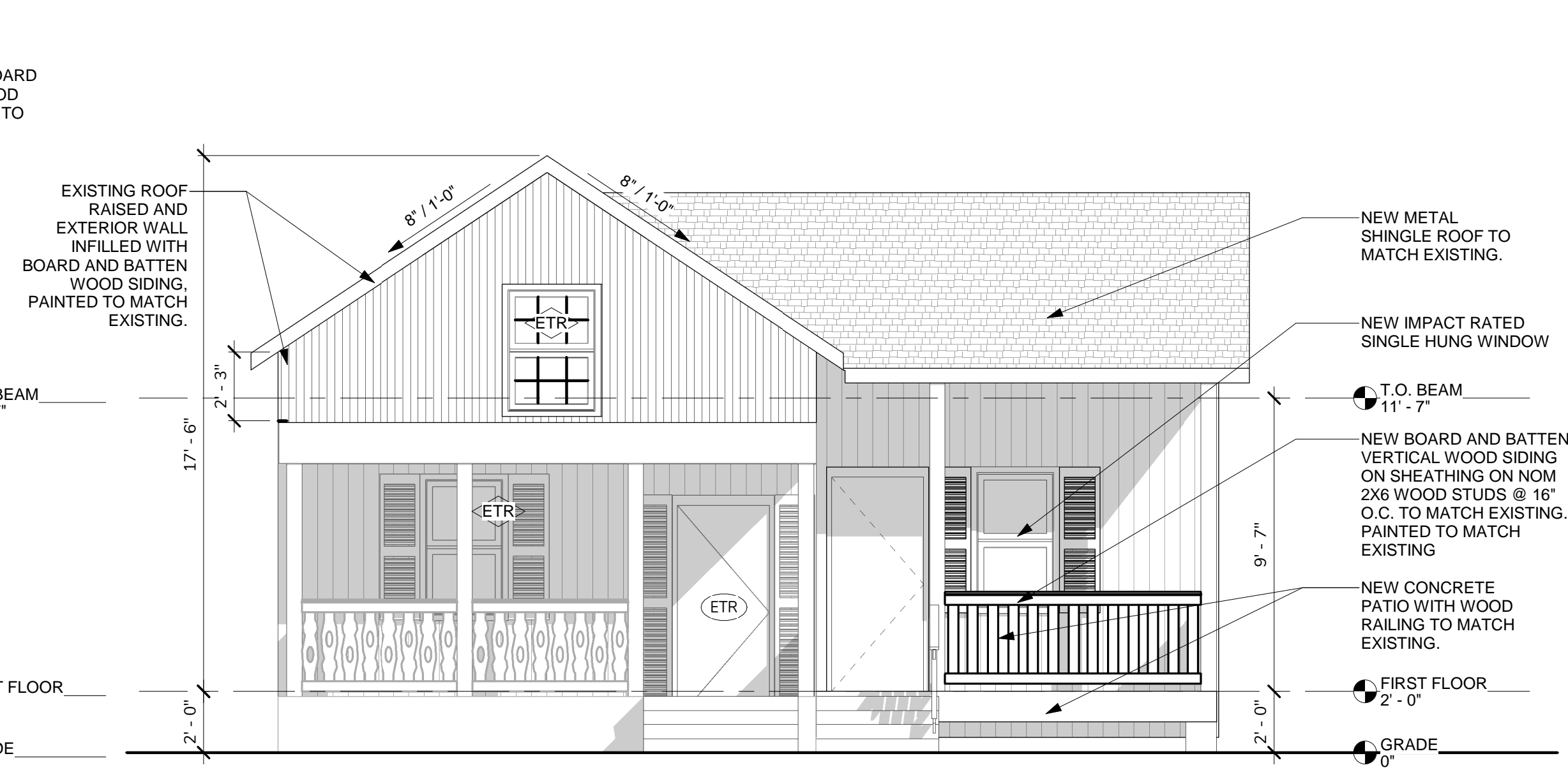
3 NORTH (FRONT) ELEVATION SCALE: 1/4" = 1'-0"
