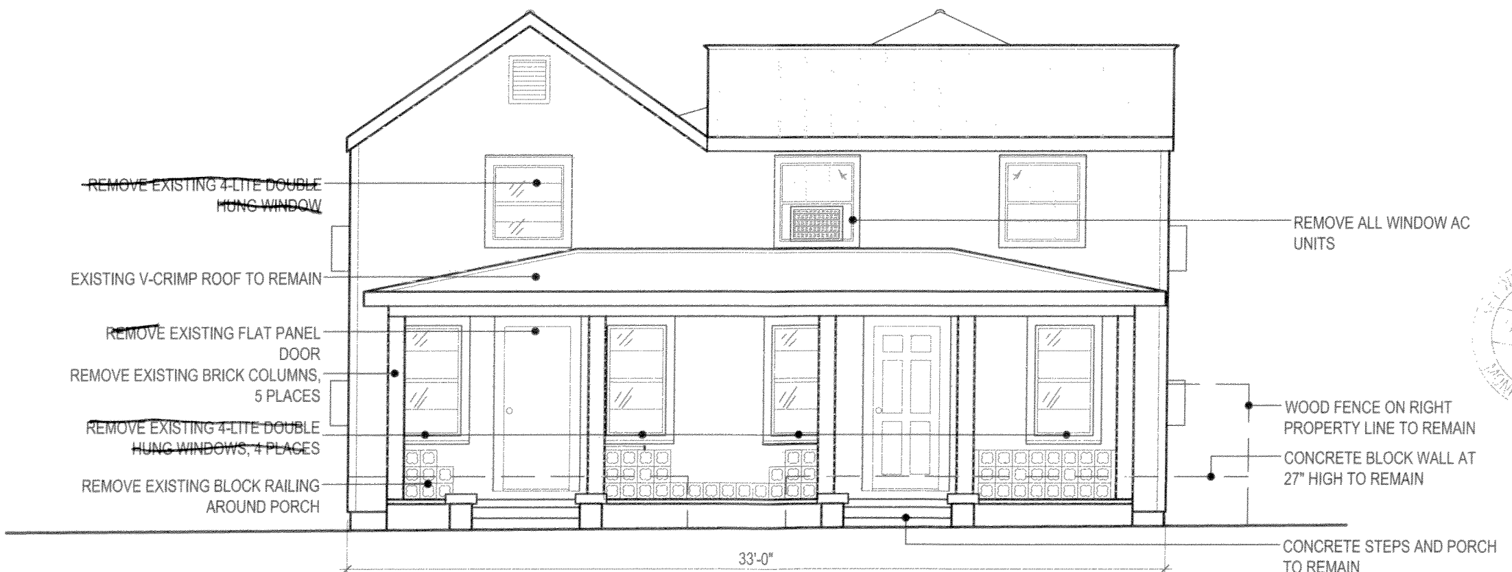
1 EXISTING FRONT (WINDSOR LANE) ELEVATION SCALE: 3/16" = 1'-0"
